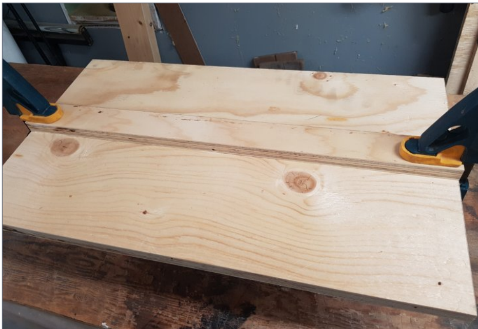
5. The module base with sub-roadbed installed.
