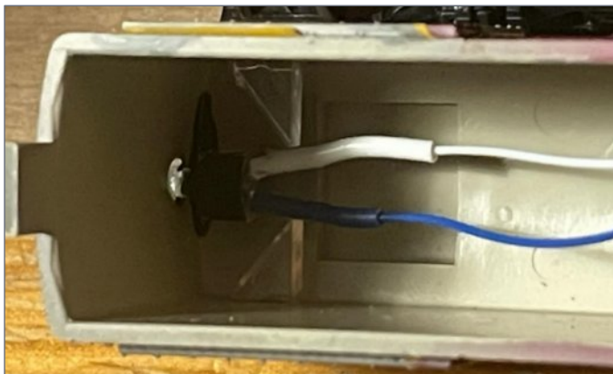
11. The front LED is in place, with the portion in the shell painted black to avoid light leak.
