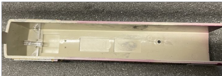
10. Headlamp and number board light pipes.
