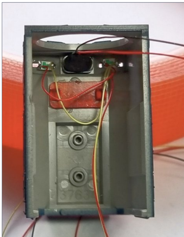
12. Rear headlight and number boards LED installation.
