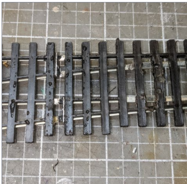
22. Jumper bars soldered in place between the closure rails and the stock rails using the 3/64" rod.
