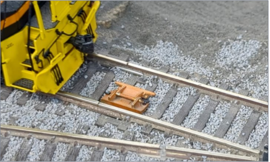
5. Derail in open position.
