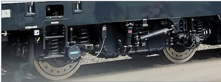
42b. Siemens-Mobility SF4 truck under an ACS-64 Amtrak Cities Sprinter. The SF4 was also used on the ALC-42 and SC-44 Charger locomotives. Note the shock absorber linked to the body.
