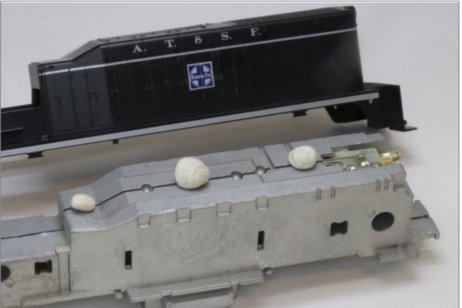
4. I applied blobs of adhesive putty along the top of the weight.
