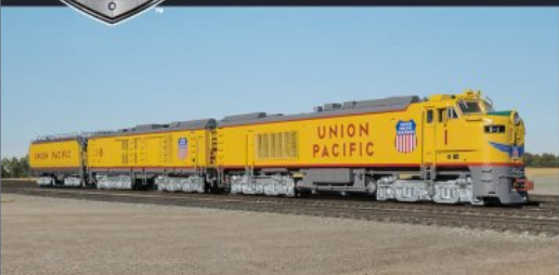
GE 8500 HP "Big Blow" Turbine
