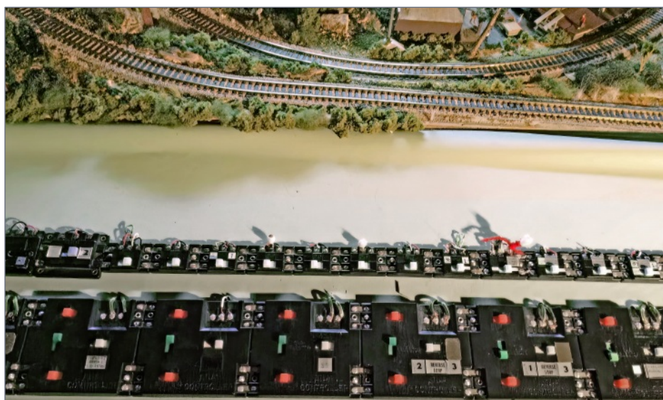
2. Atlas control panel.
