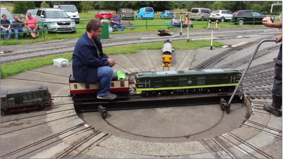
5. A large C-C locomotive takes a ride on the manual dual-gauge turntable.
