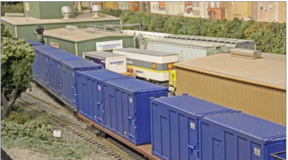
11. Municipal solid waste is a new unit-train commodity that has developed in the last 15 years. Easily identifiable by the tall, oversized containers, MSW trains can be found wherever local landfills can no longer handle the local waste.
