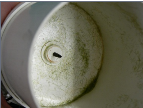
11. The ion brush in the grass chamber. Note this is NOT attached to the metal screen cap.
