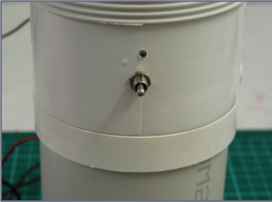
9. The switch and LED in place.
