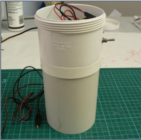
10. The unit showing the ground wire opposite the switch.
