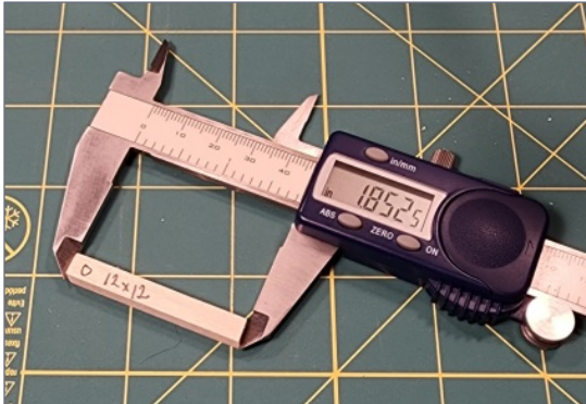
15. Measuring the cuts using a digital caliper.
