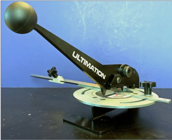
7. Ultimation Slicer with adjustable stop arm installed.
