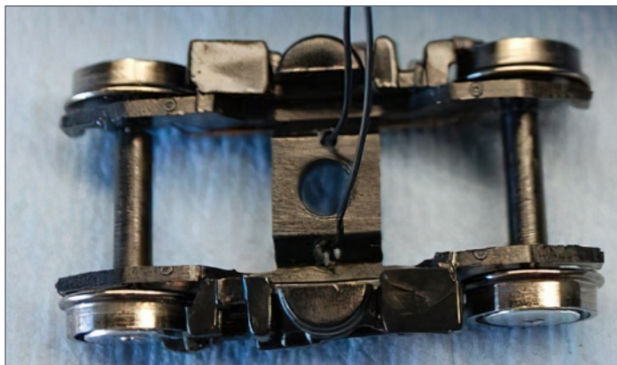
5. Truck hole positions with electrical wire pickups shown.
