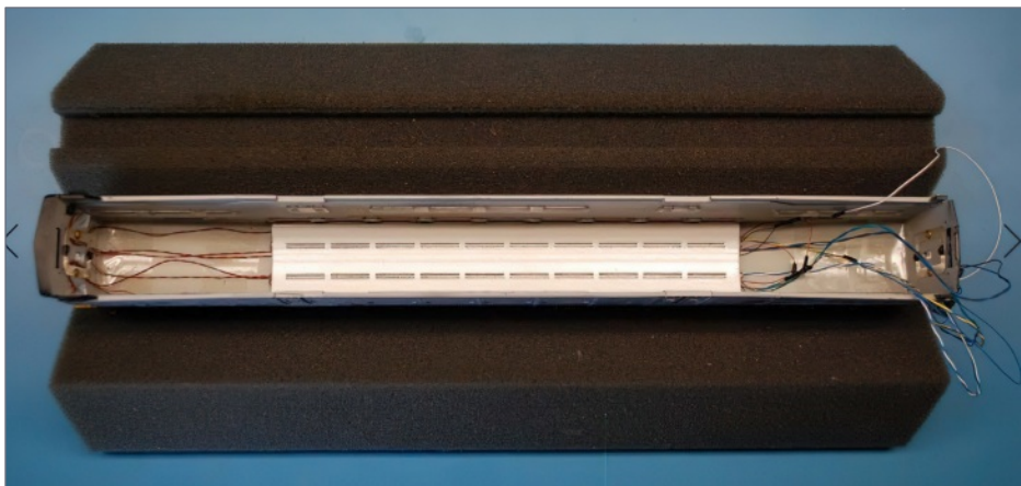
37. Upper-level light fixture installed in shell.
