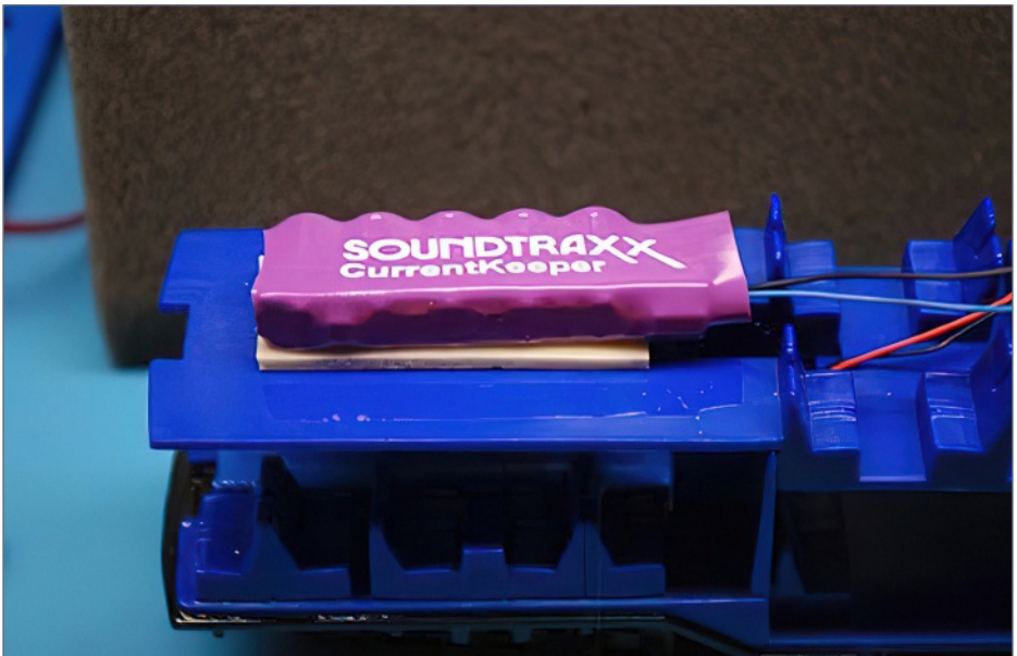
18. Current Keeper wire extension and placement.
