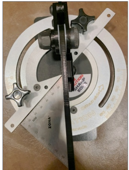
11. Testing the 45-degree angle with my Zona Triangle.
