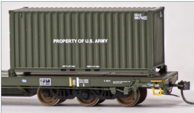
4. This picture shows the 20' Conex seated in the container cleats and the Ellcon Model 7900 hand brake lever on the Ortner car.
