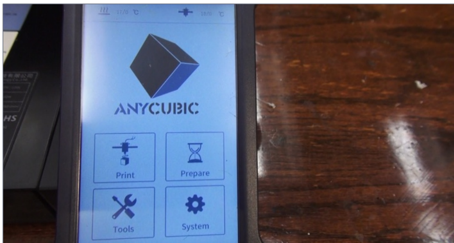
14. An LCD screen is used to control the printer, from auto-leveling the bed to selecting the file to print.
