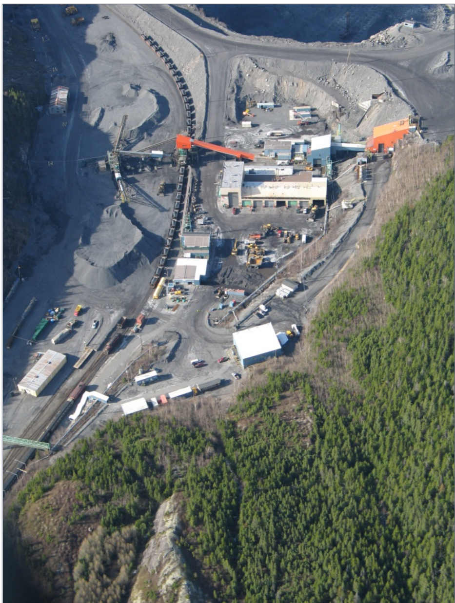
12. An overview of the mine loadout and facilities at the open pit. A loaded ore train and a lone RS-18 give scale.
