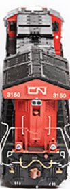
CN ET44: front &amp; rear operating ditch lights and red DPU lights
