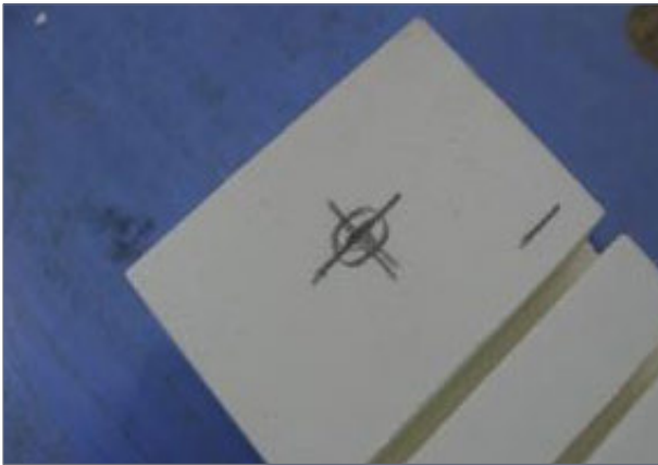
13. Mark location for mounting screw.
