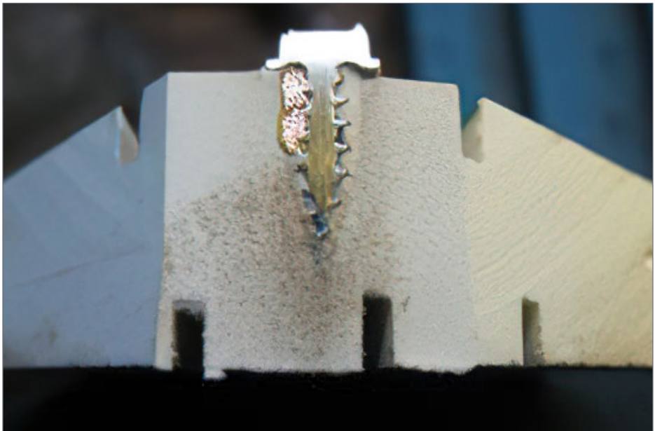
3. Cross-section through wires and the screw.
