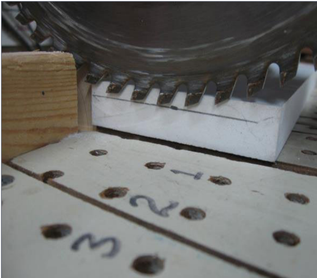
9. Cutting 12" strips from stock PVC board.
