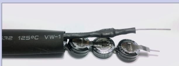
23. Shrink tubing installation.
