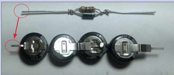
14. Solder the end of the resistor/diode assembly to the capacitor bank as shown.
