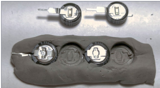
7. Use modeling clay to hold the components in place while soldering.
