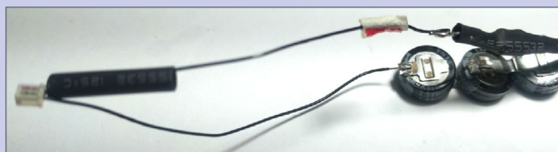
22. Installation of the JST leads.
