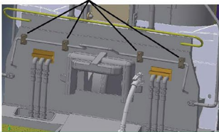
Coupler Lift Bar Brackets Plastic 2 mounting posts, .020 dia 1/32 centers
