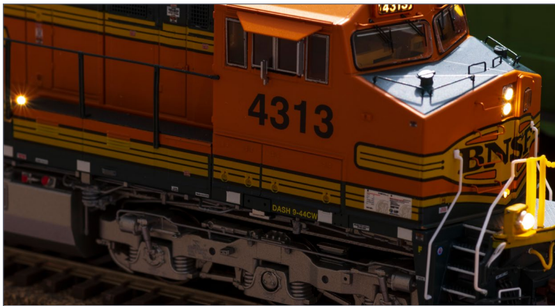
8. Illuminated number boards and front and side walkway lights.
