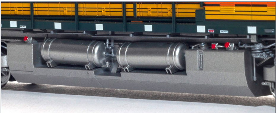
6. Close-up of fuel tank and air tank details.
