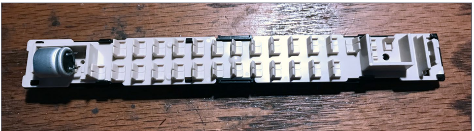
10. Capacitor placement in the car.
