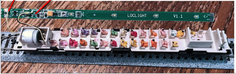
14. DR100 light board car wiring.
