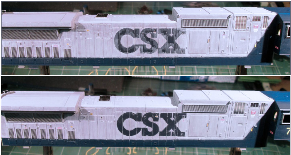
45a, b. Applying a fade coat to the gray on the long hood and subsequent cleanup.
