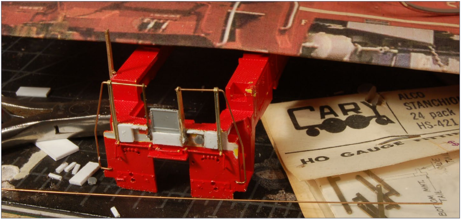
16. New front pilot details match the prototype loco.
