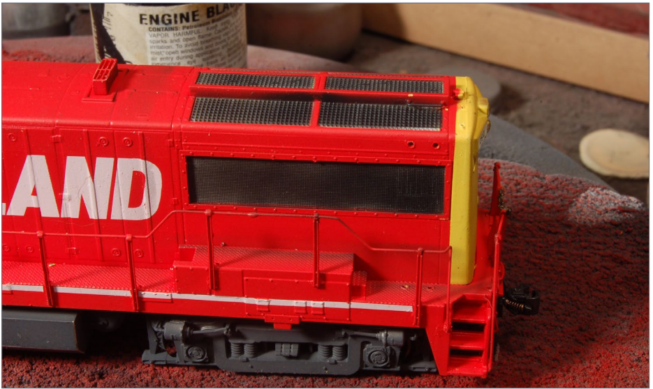
21. The finished grilles after removing the masking.
