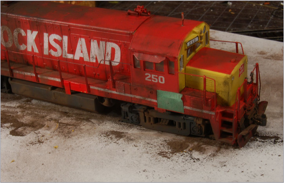
22. Weathering with Bragdon weathering powders.
