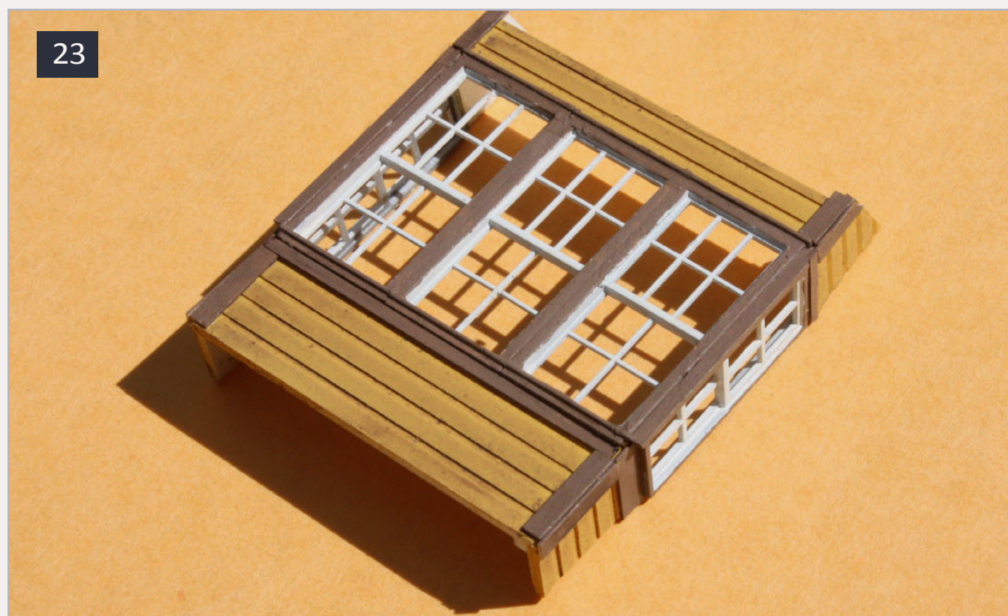
23: This shows the completed bay window section, with all trim boards in place. This section was held back and not applied to the structure until all other work was done, to facilitate glazing.
