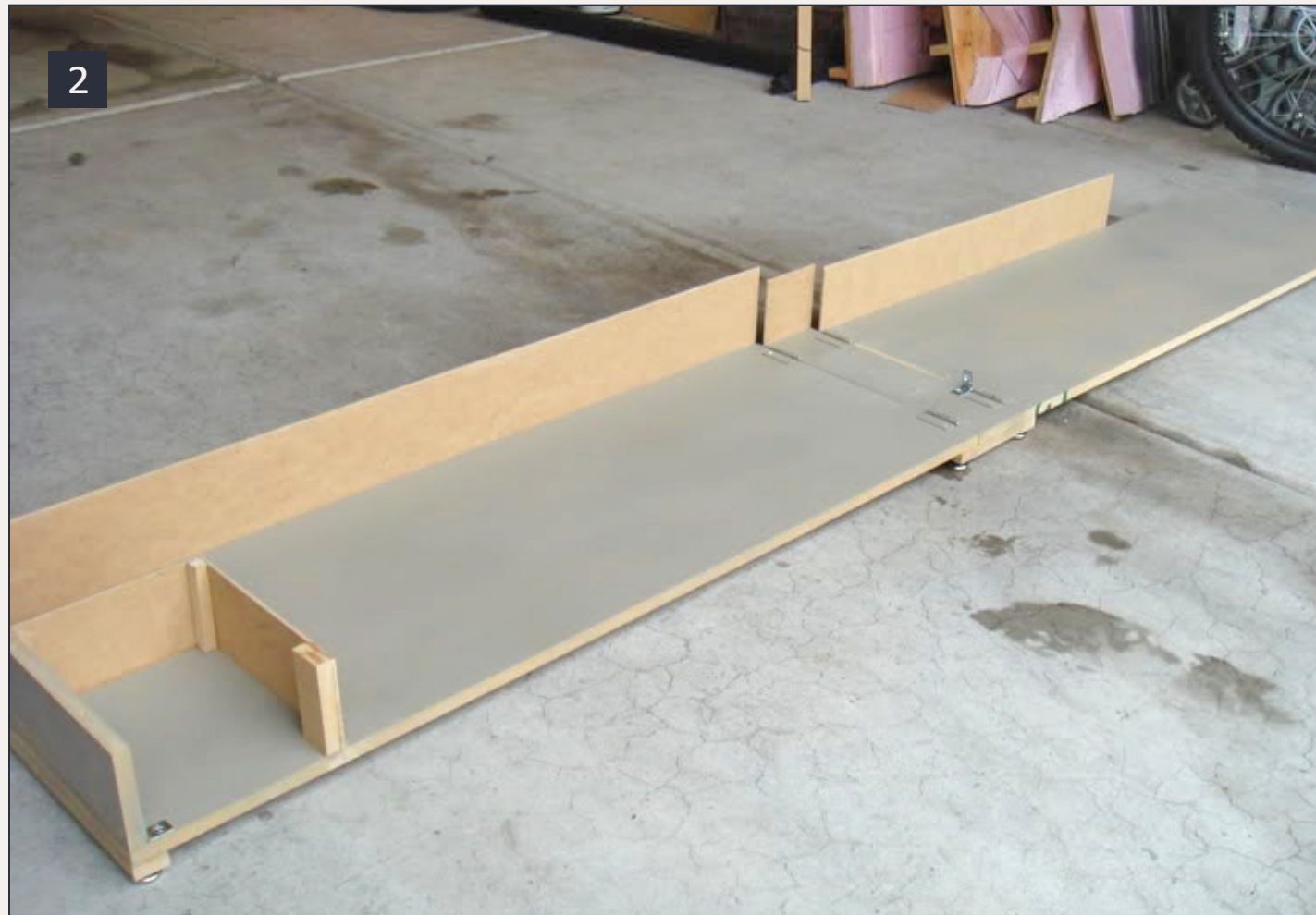
2: Here's the basic "benchwork" configuration for this shelf layout. Notice the 3" section in the middle between the two modules. In photo 4 you can see the modules folded up for transport. The 3" middle piece helps the two sections form a box, providing room for structures and scenery, yet allowing for easy transport.
