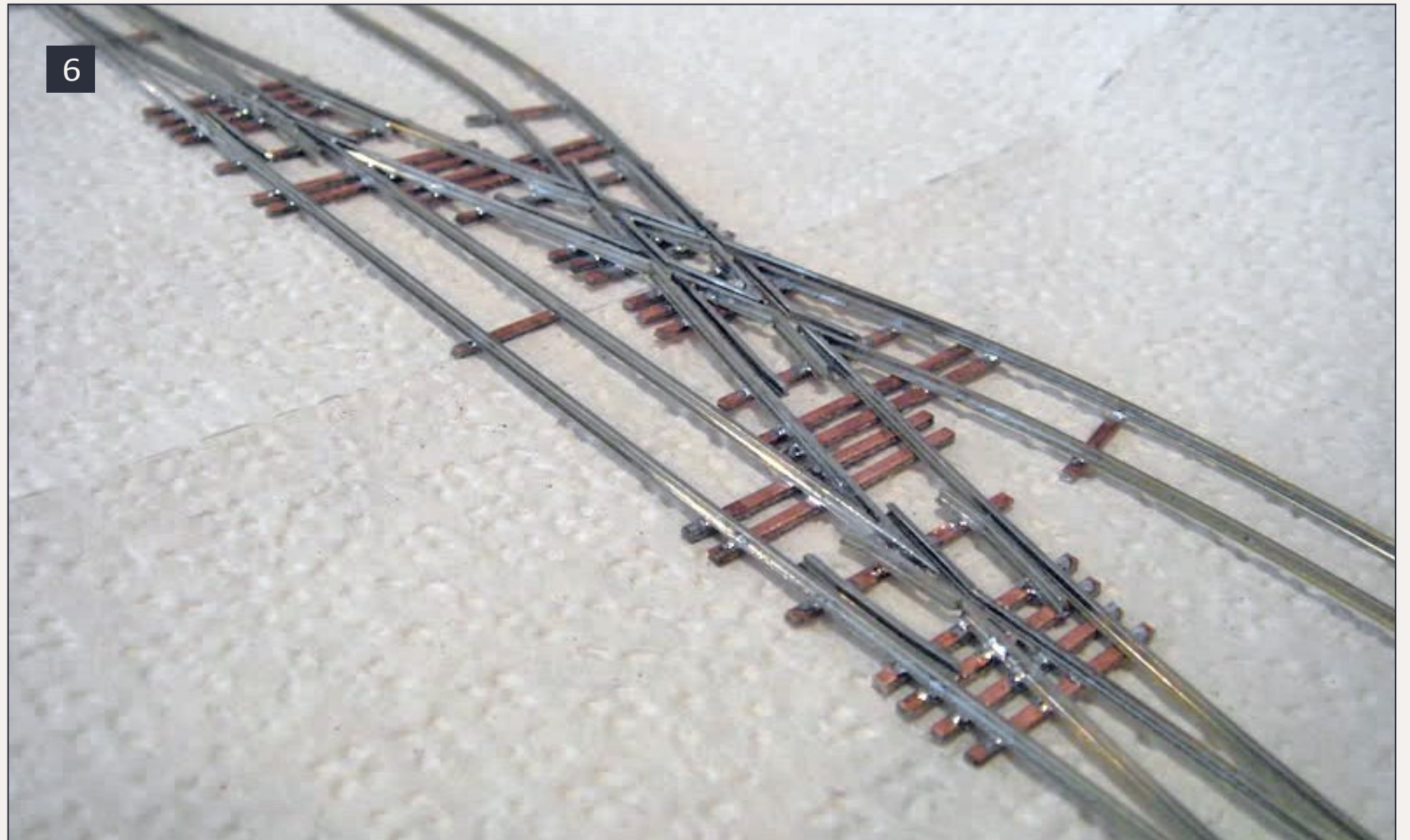
6: The addition of the brewery to Byron's original plan required a crossing between two turnouts that started curving immediately after each turnout, so I got to try out building a crossing for the first time.
