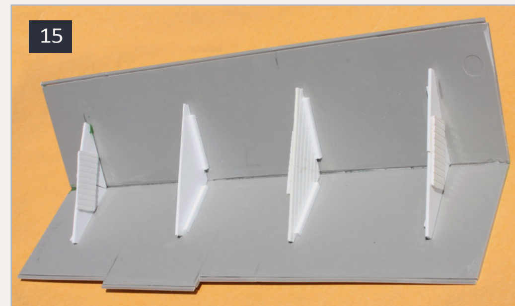
15: When the roof pieces and internal formers are assembled, adding short pieces of scale 6 x 6-inch styrene in the corners, a strong one-piece roof structure is created. The 6 x 6-inch styrene corner pieces are not visible for two of the formers, because they are on the opposite side in this view.
