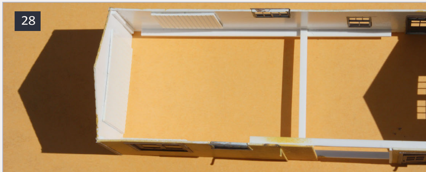
28: Interior of the completed depot, with cross-bracing to keep sides straight and all corners square. Interior corners contain scale 6 x 6-inch styrene strips. Interior partitions were added after glazing was completed. The stub downspouts can be seen on the front wall in this view.
