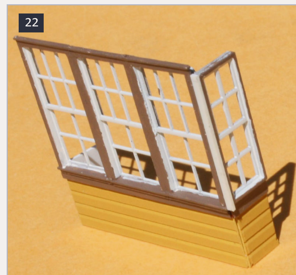
22: In this view, one side window has been glued to the bottom section, and a corner filler strip (white) of scale 2 x 4-inch styrene has been added. The filler strip will be painted brown. Trim strips below the two types of windows are 1 x 4-inch and 1 x 8-inch widths, which match up along their lower edge.
