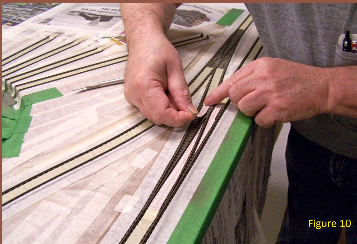
Figure 10: Using the cutouts really simplified masking the turnouts.
