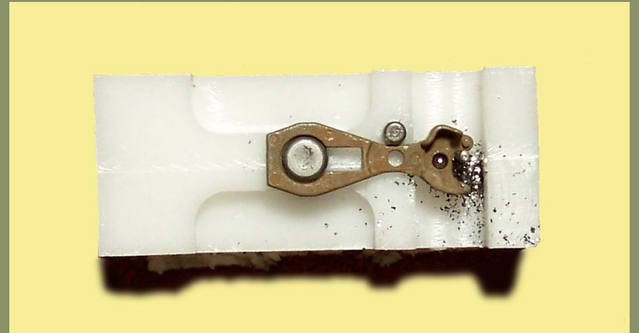
Figure 12a (Step 2): EC87K top with steel ball inserted. Sparkly stuff is Kadee powdered graphite lubricant.
