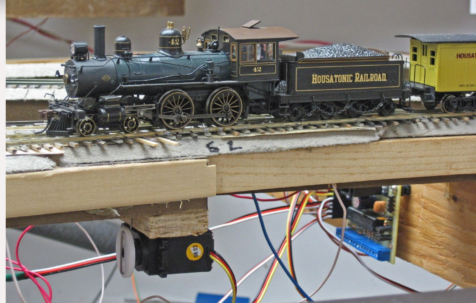
FIGURE 3: Turnout on Craig Bisgeier's Housatonic railroad powered by a servo and the original Octopus 8-servo driver. The turnout is hand-laid by Craig using Fast Tracks tools. The turnout has solid rail points, which are easily thrown by the servo.
