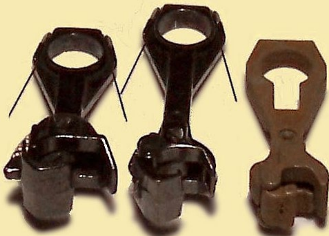
Figure 1: From left to right, a Kadee 148 “whisker” with #5 head, a Kadee #156 “long shank” with #58 head, and a Sergent EC87A.
