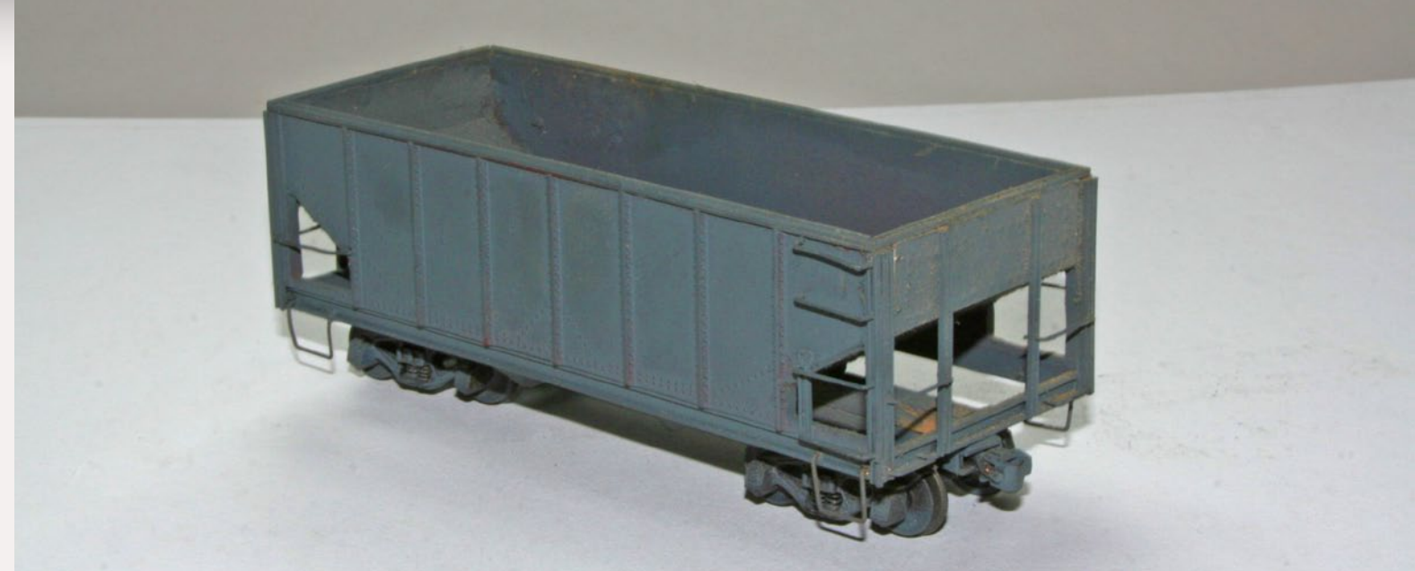
FIGURE 9: The HO car had a web on the side where the slope sheet ended at the side of the car. I chose to remove this with a file to make the side a more typical construction style. The frame was built up by adding a 1/8 inch thick piece of wood, the same width as the frame, to the top of the frame. This raised the car up just enough to be credible. Since the car has so many ribs, I considered removing every other one but the effort seemed to be too great for the small visual change. These cars should be very dirty and rusty as they are handled rough and used hard.
