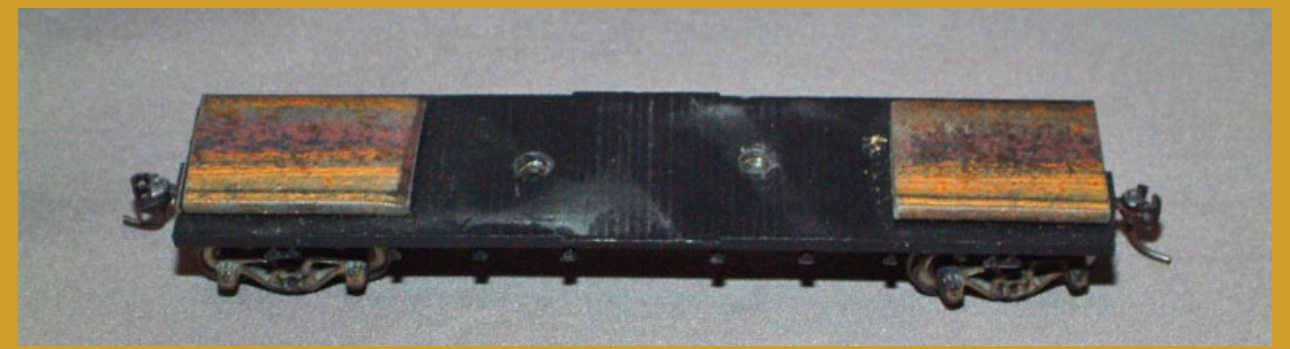
Figure 9: The car chassis, fitted with steel weights over the trucks.
