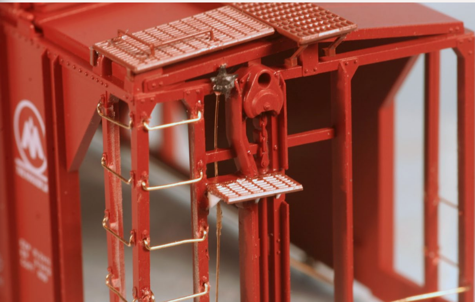
Figure 11: The Kadee Apex Tri-Lok running boards significantly improve the appearance of the roof. A bonus is that the left over material from the running boards makes a nice hand brake platform as shown. The Precision Scale Company retainer valve and .008 phosphor bronze supply line are new details not found in the original kit. These details and the wire grab irons make this model "state of the art."
