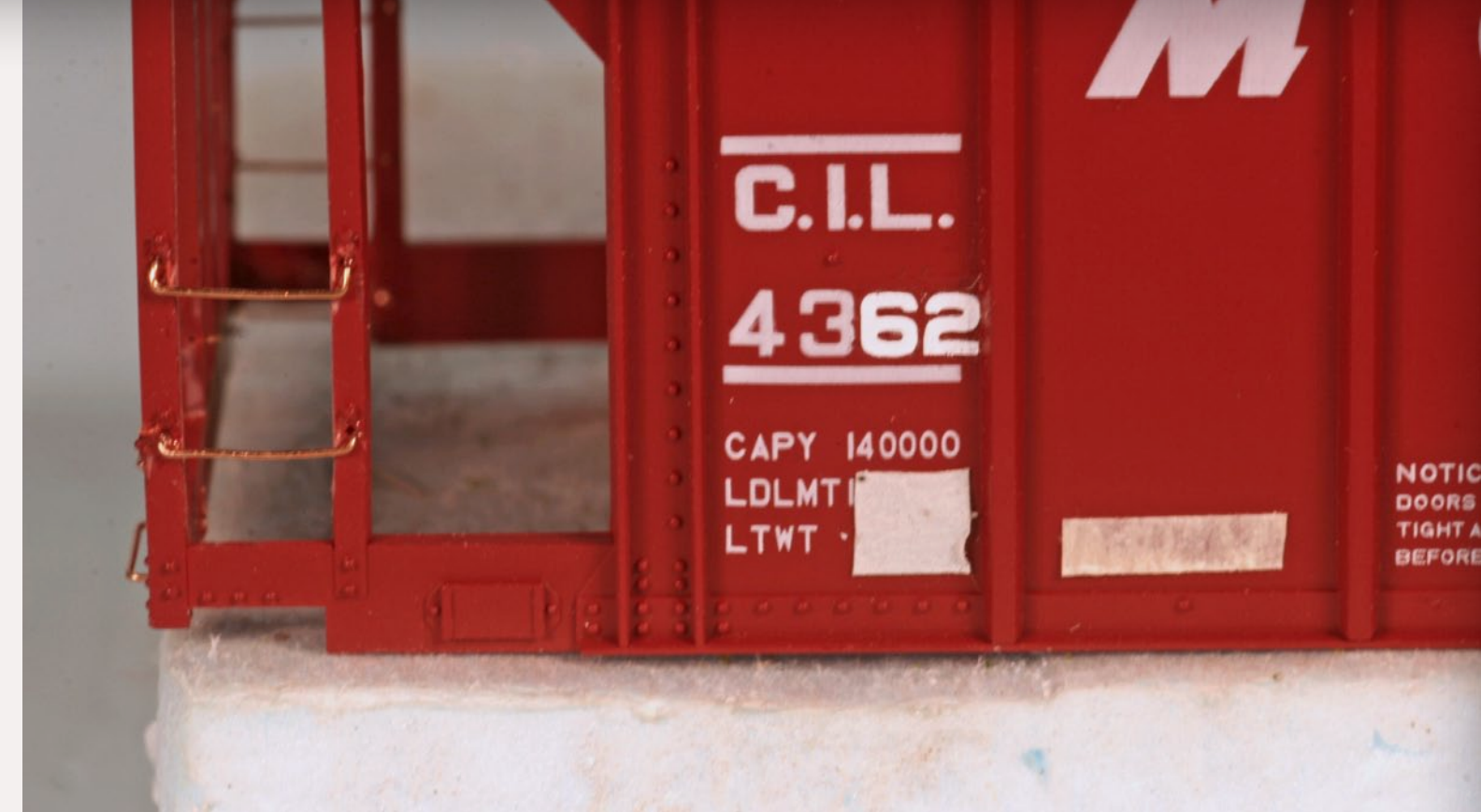
Figure 12: The car number shown here was changed by simply scraping off the factory applied number with a model knife and applying the desired number with decals. Only the last two digits of the number shown here were changed. When a car is reweighed the Load Limit and Light Weight numbers are renewed along with the location and date. Since this data was included on the factory painted model all that is required to accurately represent it was to protect it with masking tape during the weathering process.
