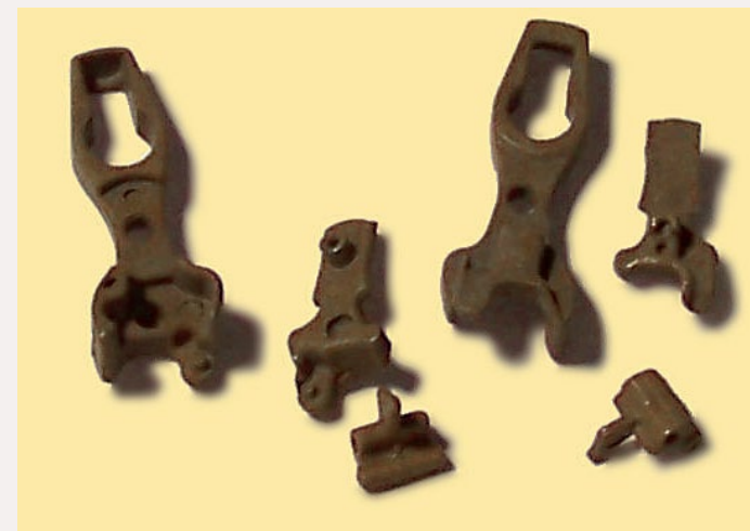
Figure 5: EN87K narrow shank couplers, pre-assembly. Pieces seen: top (with shank), bottom, and knuckle. Not shown: steel ball to lock knuckle closed and shank friction spring.
