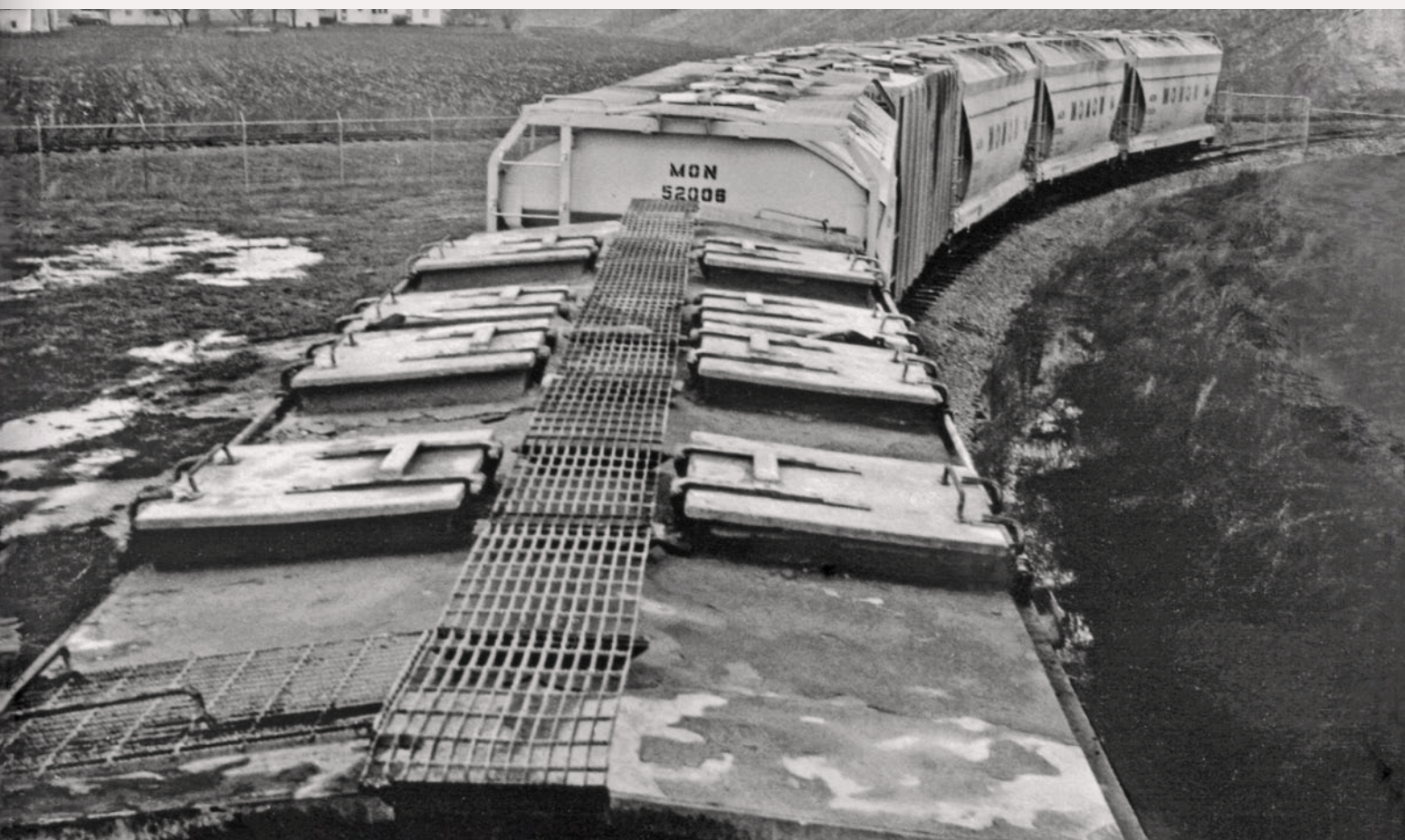
Figure 13: MON 4362 (roof view) shows that not all of the cement went into the cars during the loading process. The claws on the outer edge of the roof hatches hold them closed. When released the hatches open inward toward the running boards.
