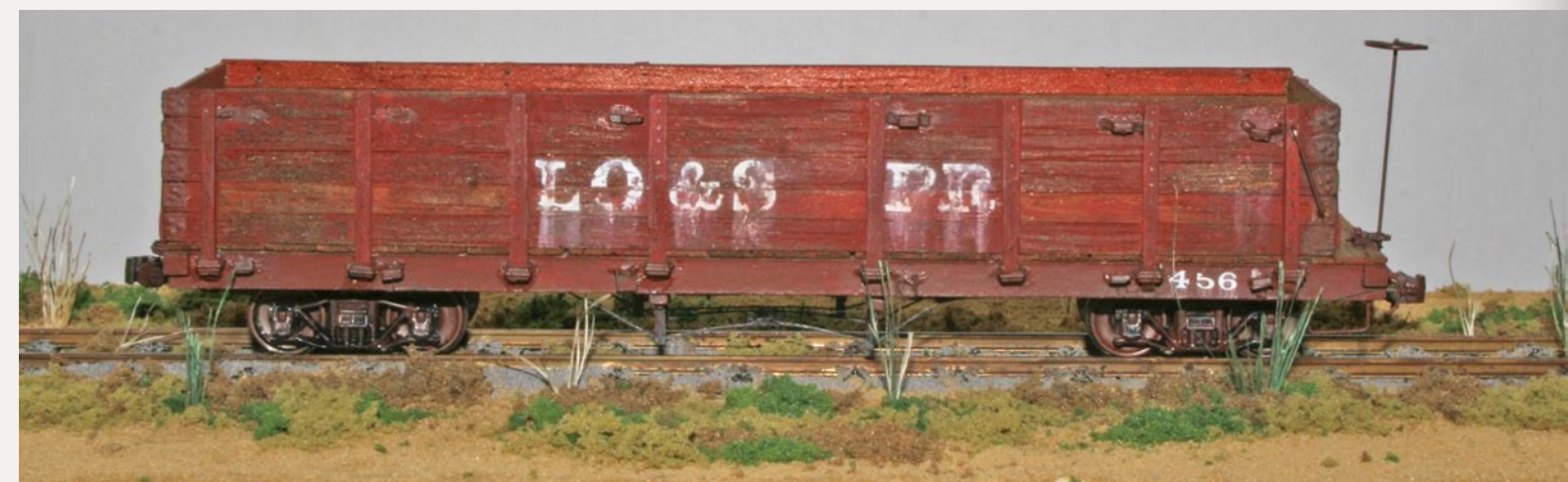
FIGURE 4: The sides of the gondola were assembled on the workbench from prestained scale lumber, model airplane style, over a wax paper protected drawing and held together with pins. Details were added, such as plastic nut bolt washer castings, card stock stake pockets and wire grabirons while the sides were laying flat. Small bolts connecting the stakes to the boards were made from dark brown ink dotted in the correct place with a #0 technical pen. The arch bar trucks shown here have HO 36" diameter metal replacement wheel sets with the code 80 semi-scale tread.
