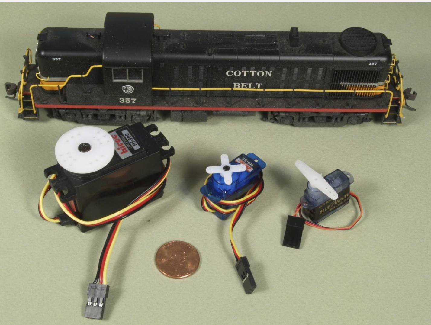
FIGURE 1: Three sizes of R/C servos with an HO scale locomotive and a penny for size comparison. From the left are a standard, mini and micro servo. All 3 servos have a standard 3-pole plug and despite their different sizes and all respond identically to standard R/C servo signals. The white servo arms can be replaced by a wide variety of different size and shapes for connecting to different devices. In this article I show a few uses for model railroads including turnouts and semaphores.
