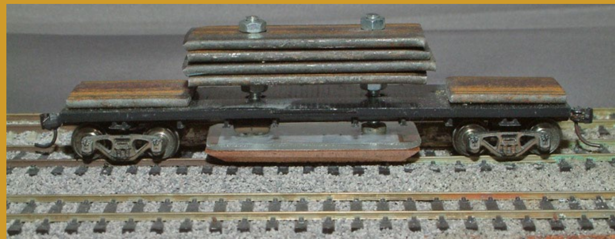
Figure 12: The weights mounted on the pad threaded rods and secured with two more nuts.
