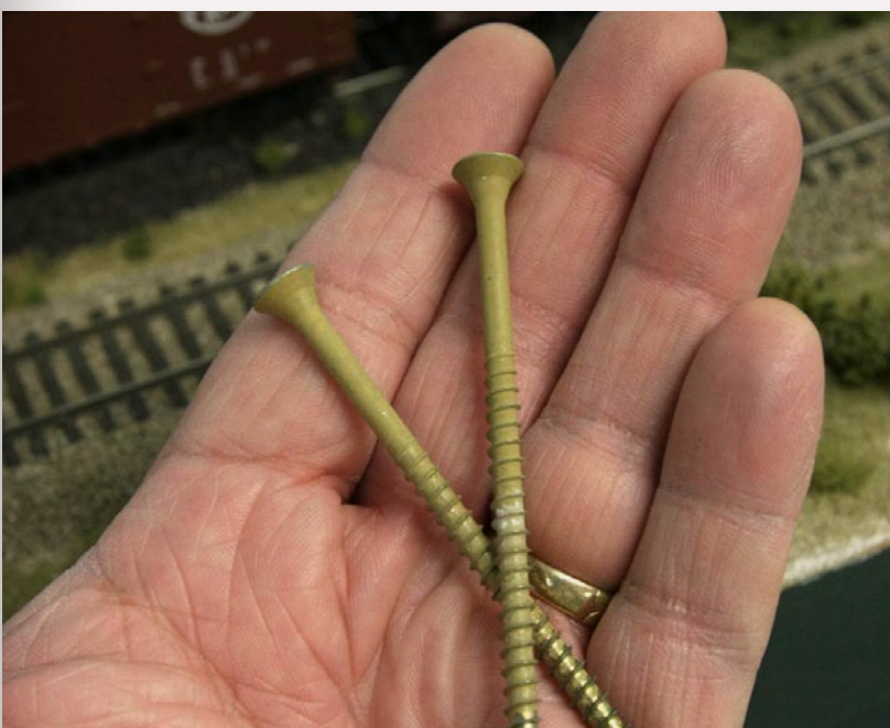
FIGURE 1: 3" deck screws securely fasten cleats to 2x4 wall studs.
