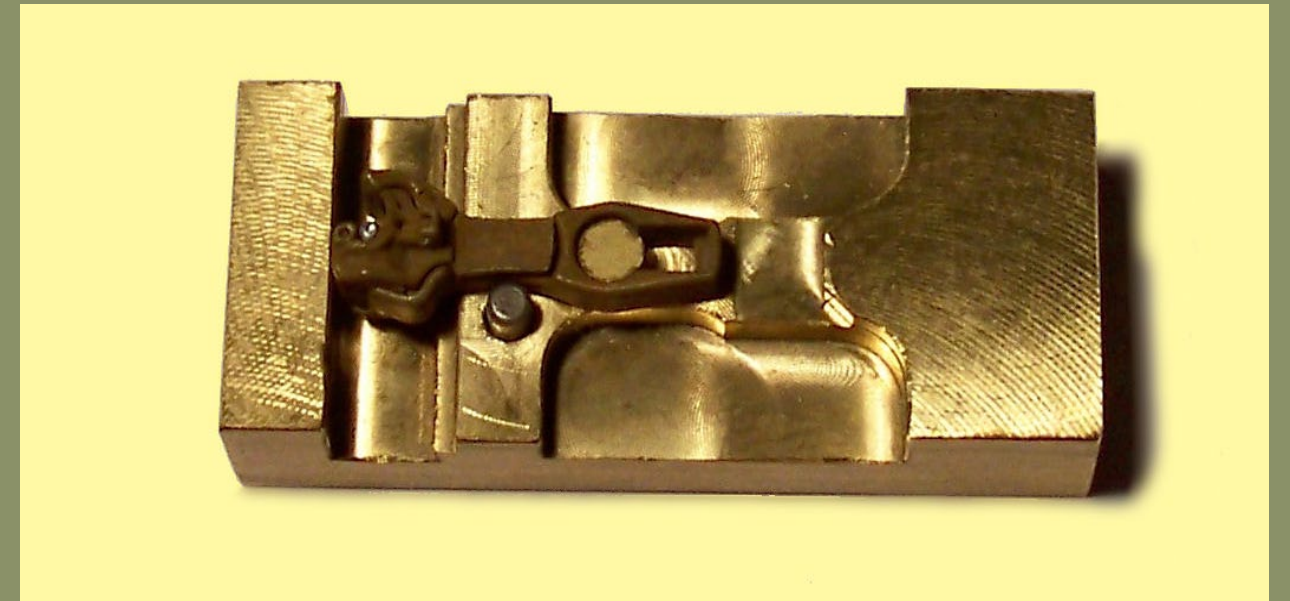
Figure 11c (Step 3): EN87K completed coupler with bottom plate CA'd on.
