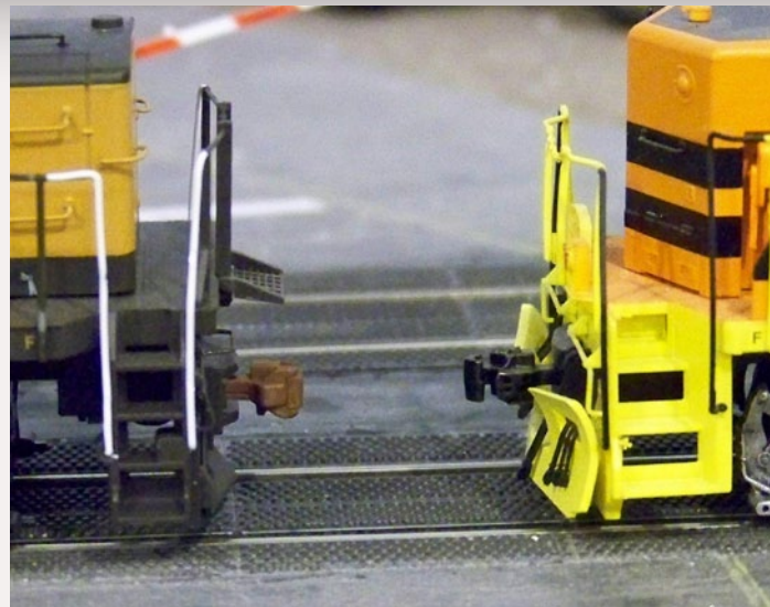
Figure 8a: Kadee #148 coupler (right) in an Atlas GP38 and EN87A coupler mounted in an Atlas C425 (left).
