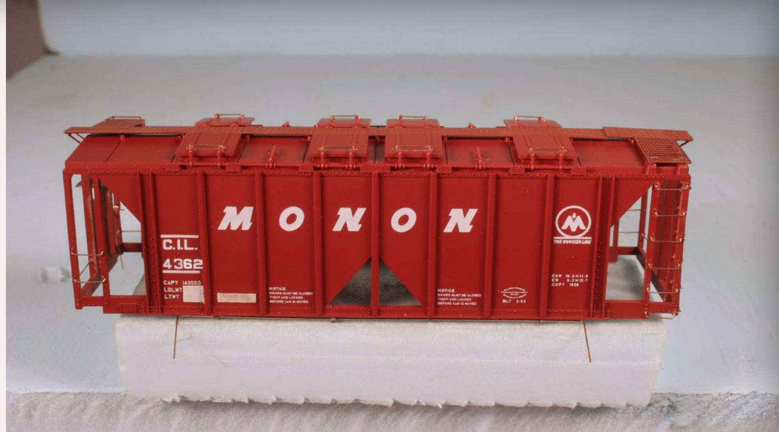
Figure 8: The train air line runs along the right side of the car when facing the "B" or brake end. The air line is made from .0125 phosphor bronze wire and is held in place with Athearn handrail stanchions. Small eye bolts can be substituted for the stanchions.
