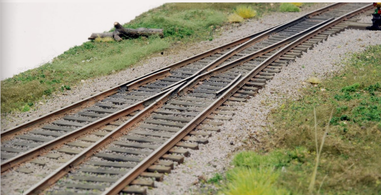
FIGURE 5: Using a Floquil Paint Pen, rust color, on the sides of the rails is quick and very easy to do with this product. The results are dramatic and add a very realistic touch to any finished trackwork.
