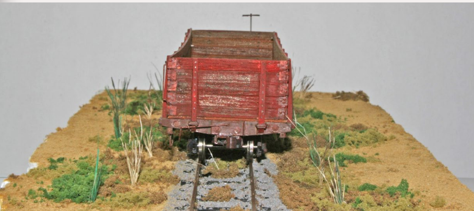
FIGURE 2: The boards on the end were stained and painted individually before construction to ensure randomness in the color. Note that the brake airline hose has yet to be installed.
