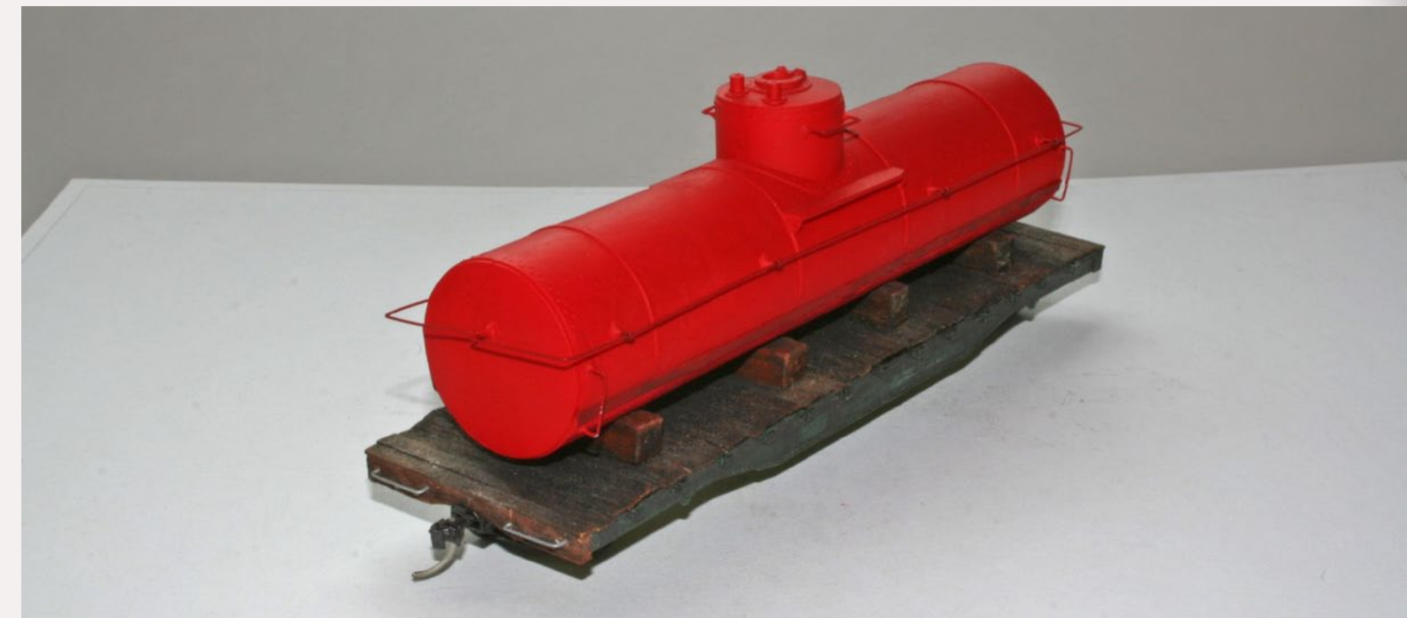
FIGURE 13: The tank car built on a flat car represents about a 6,000 gallon car. This type of car could be used to haul on-line lubricants and diesel fuel, even perhaps, gasoline. I will place this car, when completed, as a static model at a siding with a fuel depot and a tank truck or two. The hatch will be open showing the valve inside the dome and a discharge hose will come from the bottom of the car and go into the underground fuel storage area. Adjacent tracks will hold cars for operations.
