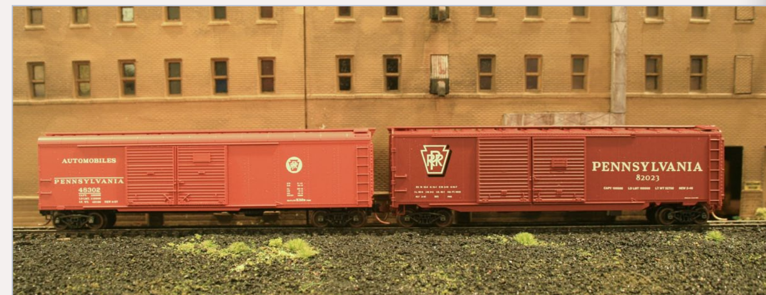
FIGURE 5: Two M-T 50-foot boxcars; the round roof X32B and double door X41.
