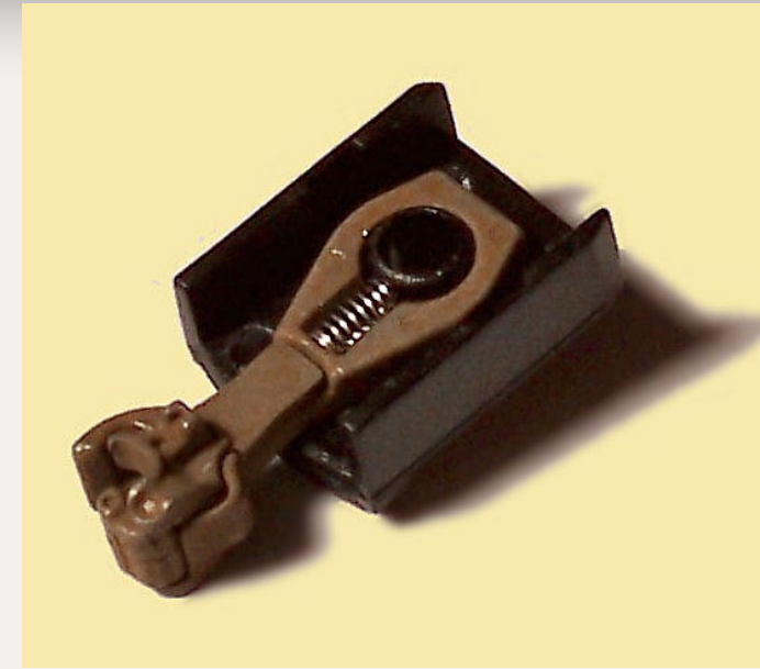
Figure 4: EC87A compatible width shank from the bottom, mounted in an Atlas locomotive coupler box.
