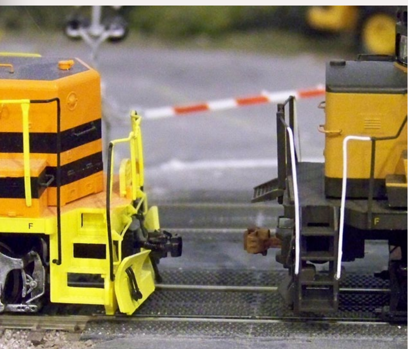
Figure 8: Kadee #148 coupler (left) in an Atlas GP38 and EN87A coupler mounted in an Atlas C425 (right).
