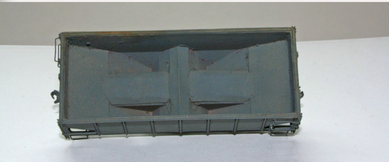
FIGURE 8: You can see on the inside where the car was widened along the centerline axis and the cut covered with cardstock pieced over the slope sheets and frame. When the car is loaded with a coal covered foam rubber insert, none of the interior detail is visible and the frame doesn't need covered. Some people may find the width of the cover to be too wide and choose not to do the cover up this way. Detailing and weathering of the slope sheets should include some streaks of shiny steel from the scouring action of the coal as it slides down the sheet.
