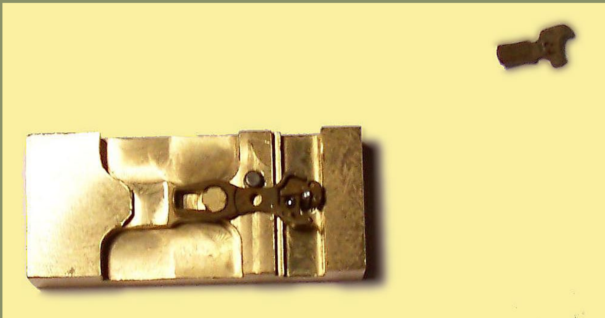
Figure 11b (Step 2): EN87K top with steel ball and knuckle in AFN coupler assembly jig.
