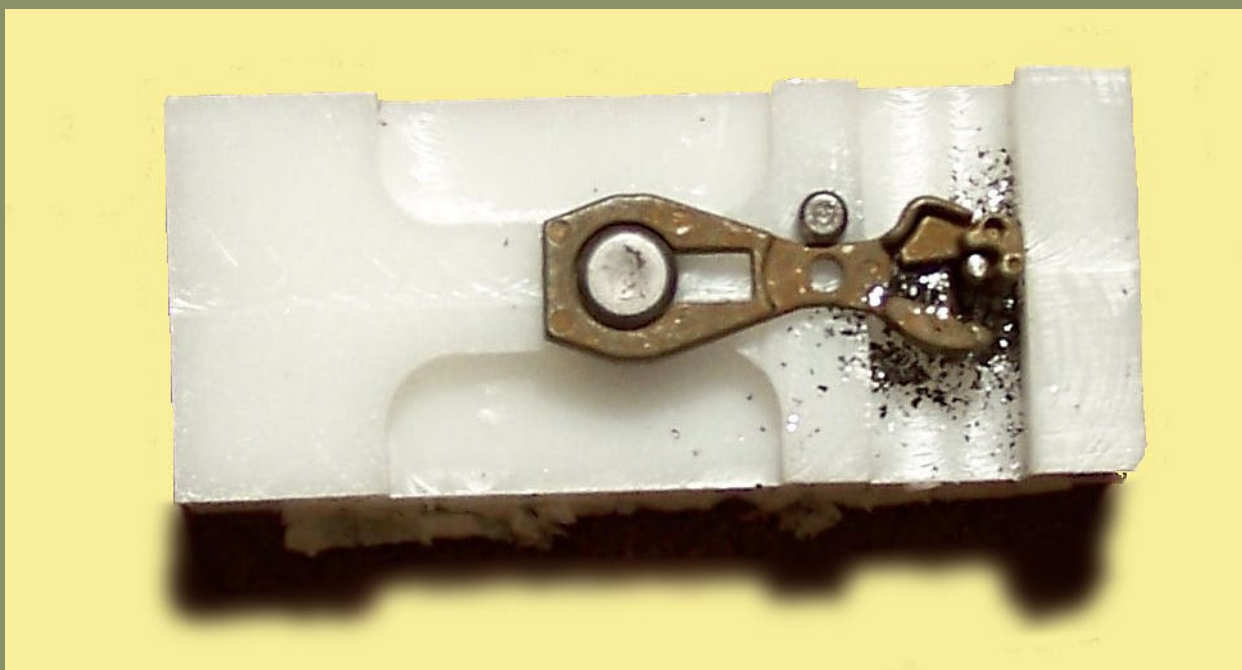
Figure 12b (Step 3): EC87K top with steel ball and knuckle.
