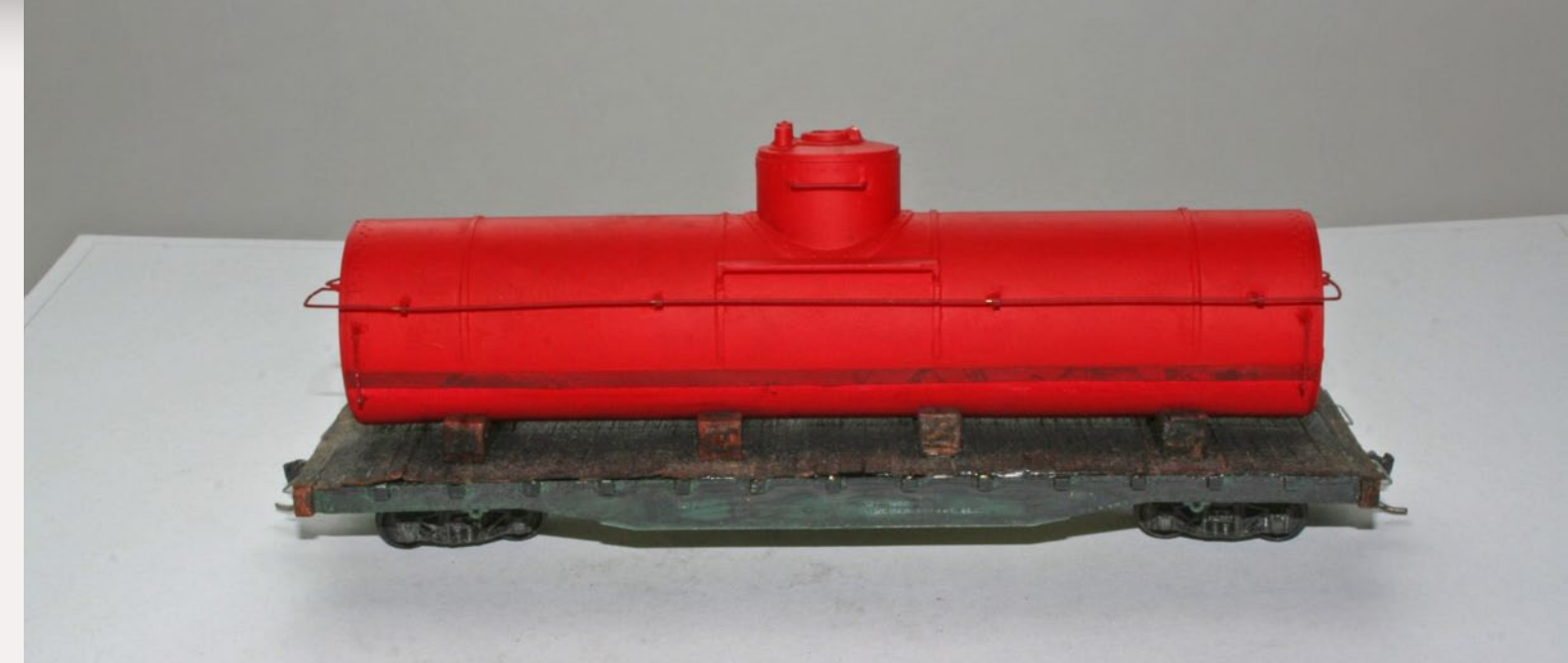
FIGURE 12: The tank car built on a flat car uses the same "flat" construction as the gondola. The length of the car is 20 feet and the tank is from a junk-box Lionel O27 trainset car. The tank, based on the venting and the horizontal courses is the style of the 1920s and newer. A very modern car.
