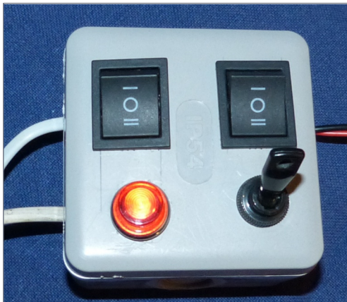
19. Control box with the two rocker switches. Each controls one pair of doors.
