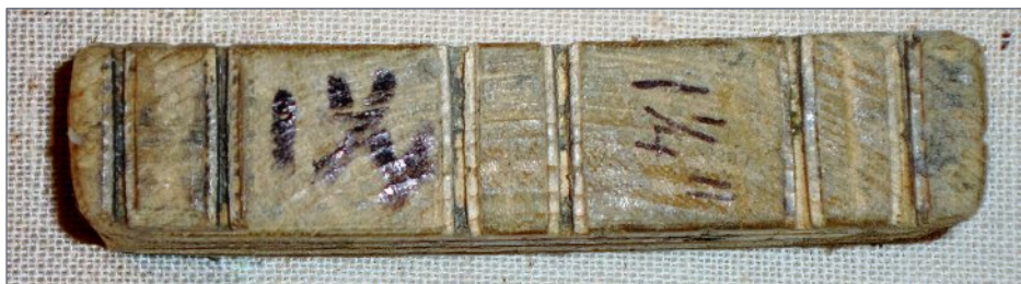
3. Straight track spacing jig for N scale using 1-1/4" separation.
