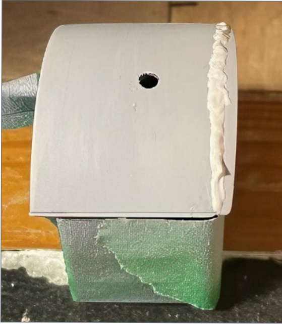
4. The first layer of primer revealed unacceptable putty lines.
