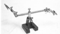
[6-4] A so-called "third hand" is infinitely handy for holding wires or parts being soldered or glued together.
