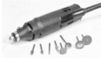
[6-3] You can hardly get by without a Dremel-style hand tool and an assortment of cutting, grinding and polishing bits.
