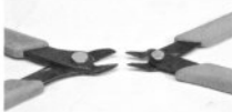
[6-5] Xuron Rail Nippers are fantastic tools for making clean, flush cuts in soft metals such as brass or nickel silver. Don't use the Rail
