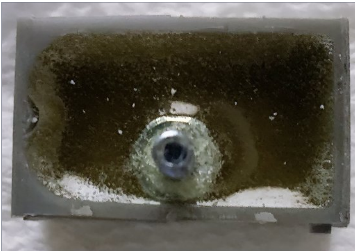
20. Screw is placed and epoxy poured.
