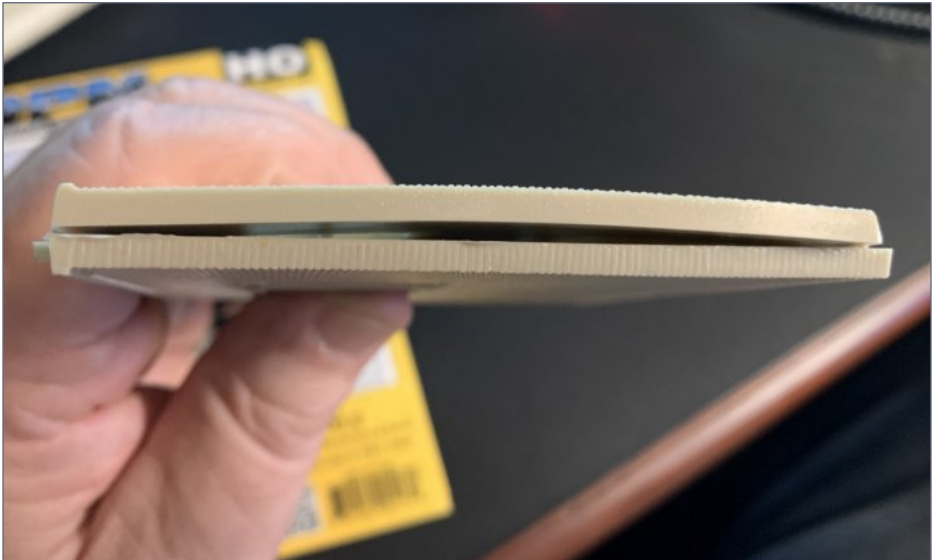
5. The back wall had a significant bow.
