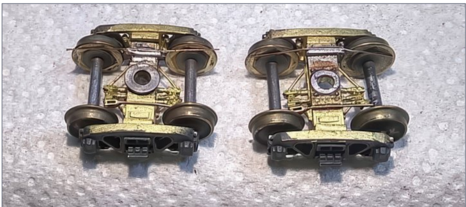
13. After soldering the wire wipers, I bent them to make contact.
