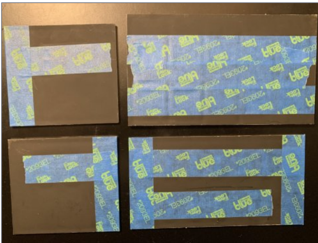
13. The interior window openings and glue edges are masked.
