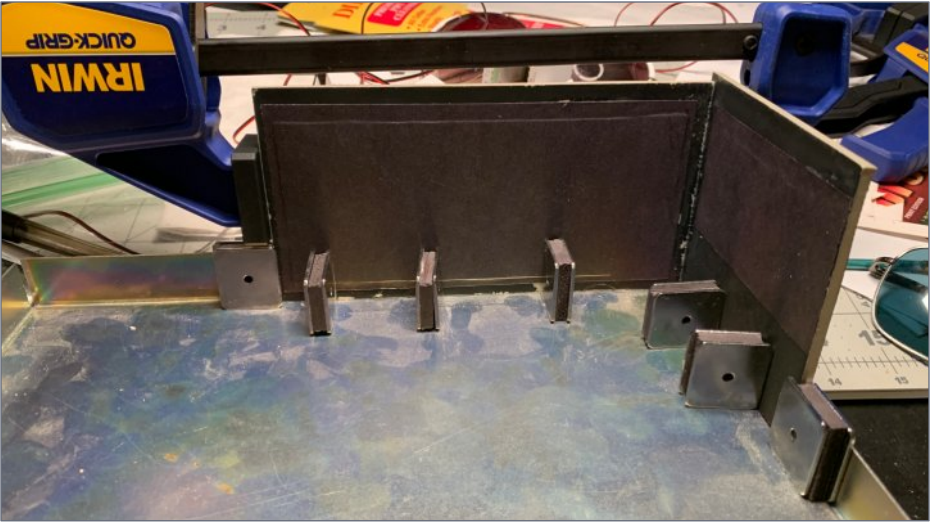
21. The first two walls assembled. The magnets hold the walls in square against the frame. A clamp adds reinforcement to the joint.
