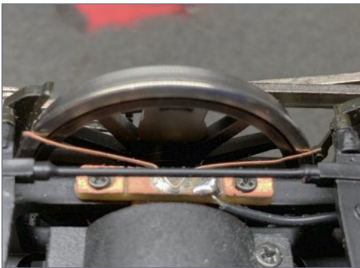
8. The replacement driver retainer plate made from PCB stock.
