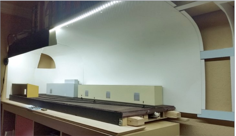
34. The matte board curved nicely on the new backdrop framework. There is one triangular corner area I filled in.
