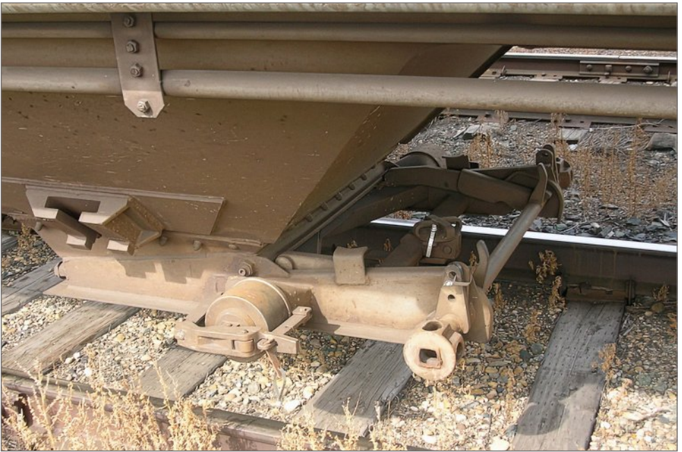
2. Closeup of the pneumatic doors on a subset of the hoppers.
