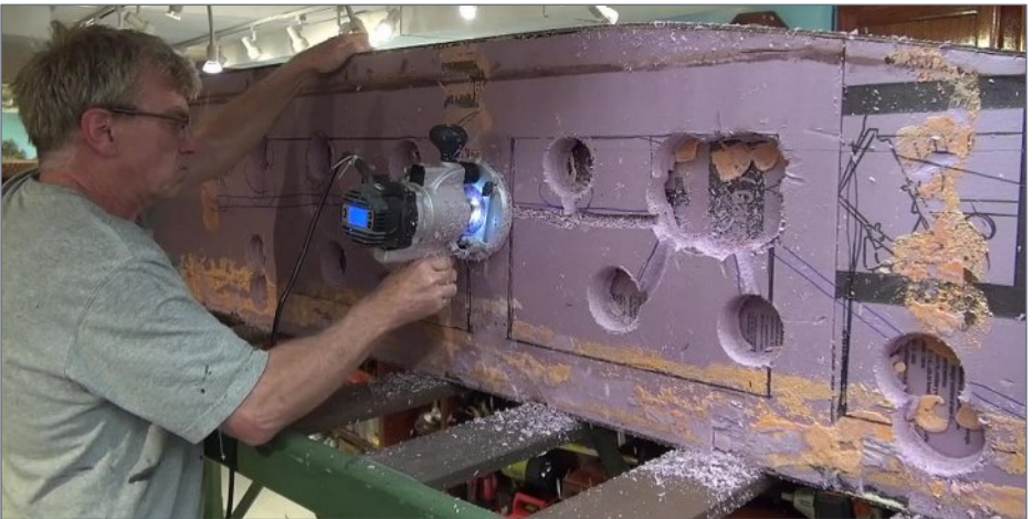
11. Having marked where he wants to install the Atlas 30-foot double- and single-head lights, Ken flips up the diorama to access the underside, using a hole saw to go through the bottom foam layer where the lights will be, and then using a router to remove the foam for the wire paths.
