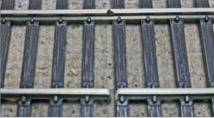
24. While making the cut in [23], the opposite rail was nicked.
