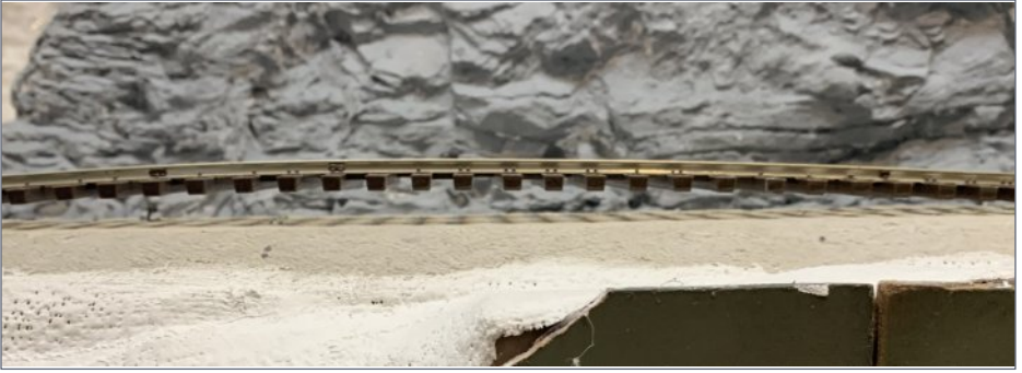
28. Heat expansion differences between the road bed and the track caused the track to bow up.
