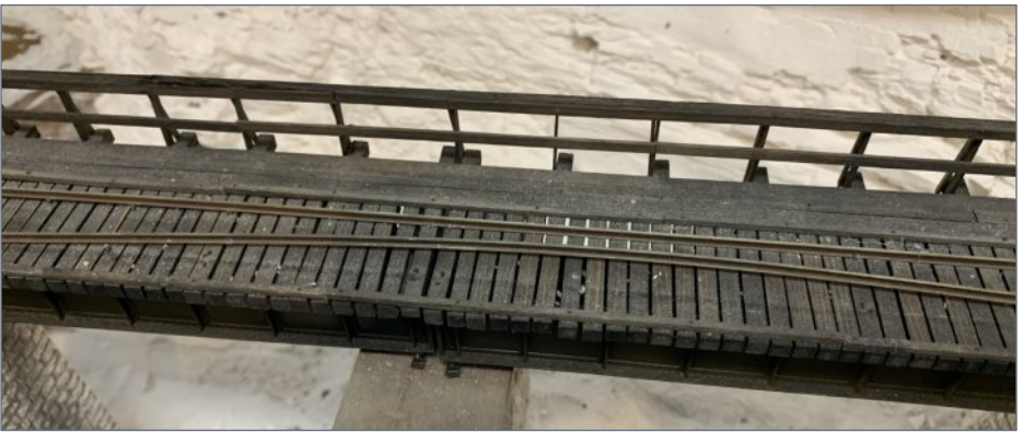
29. Heat kinks have bent these rails out of gauge.
