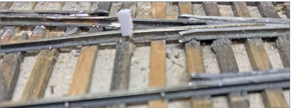
26. This piece of plastic has been rough-cut to fit the gap.
