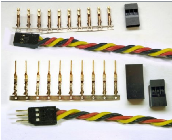
9. Here's what comes in the kit. Note that we use the plug with the tab on the side for the male pins.
