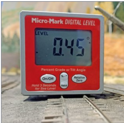
6. A digital level such as this one from Micro-Mark can offer an exact measure of slope angle in degrees or as a percentage of grade. Here, the level shows the rails are 0.45 degrees off level, with the right rail higher than the left.
