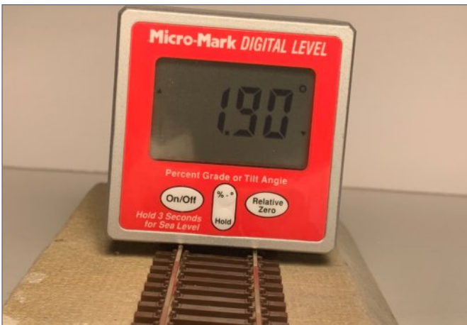
9. The track level shows a tilt of 1.9 degrees, enough to cause trouble.
