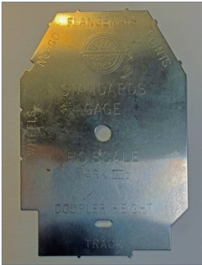
5. The NMRA standards gauge is an excellent tool, but it doesn't tell the whole story, especially if it's a leveling issue.
