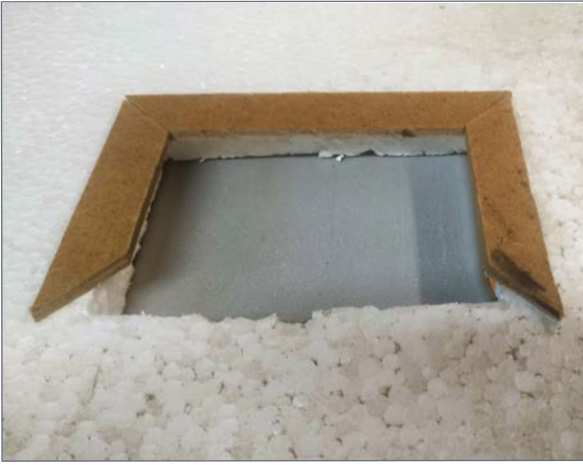
10. Masonite lip around cutout in baseboard, viewed from under the layout.
