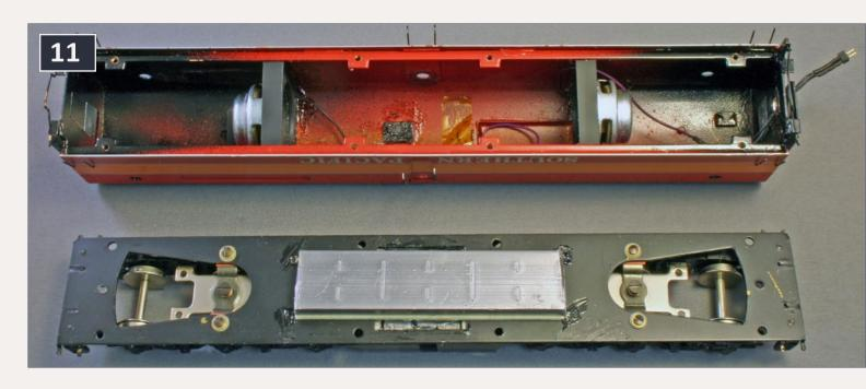
11. Westside Alco PB with an enclosure set up with 28 mm high bass speakers.
