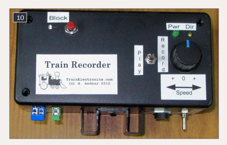
10. This is yet another unit with simplified controls. Speed is adjusted with the knob on the right. The larger green LED shows the power level, and the smaller LED next to it indicates direction. The Play/ Record switch is to the left of the speed control. The LED and switch in the upper-left are for the block sync relay. When the relay is active and the block is unpowered, the LED is lit.
