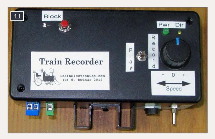
11. This side view shows the power connections and on/off switch on the right. The track is connected to the two blue terminals on the left. The cut section of the block is connected to the single green terminal.
