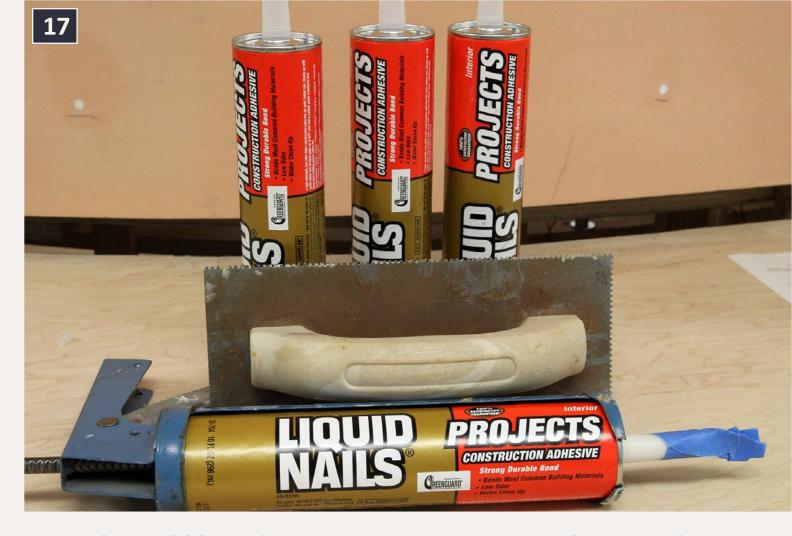
17. Liquid Nails for projects cleans up with water, has no nasty solvent vapor outgassing, and gives me up to 15 minutes to get the layers clamped. I was amazed at how much adhesive it took for each 4x8 sheet – at least two tubes. The trowel has 3/32" notched edges.
