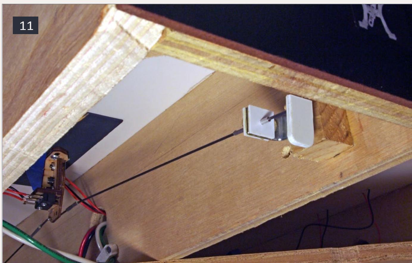
**11: I prefer manual turnout control, so I assembled and installed a Fast Tracks Bullfrog with homemade control rods made out of music wire. Given the 50” layout height and the 24”-or-less module width, the control rods are actually unnecessary as we’ve found it’s easier to just reach underneath from either side and throw the Bullfrog itself.**
