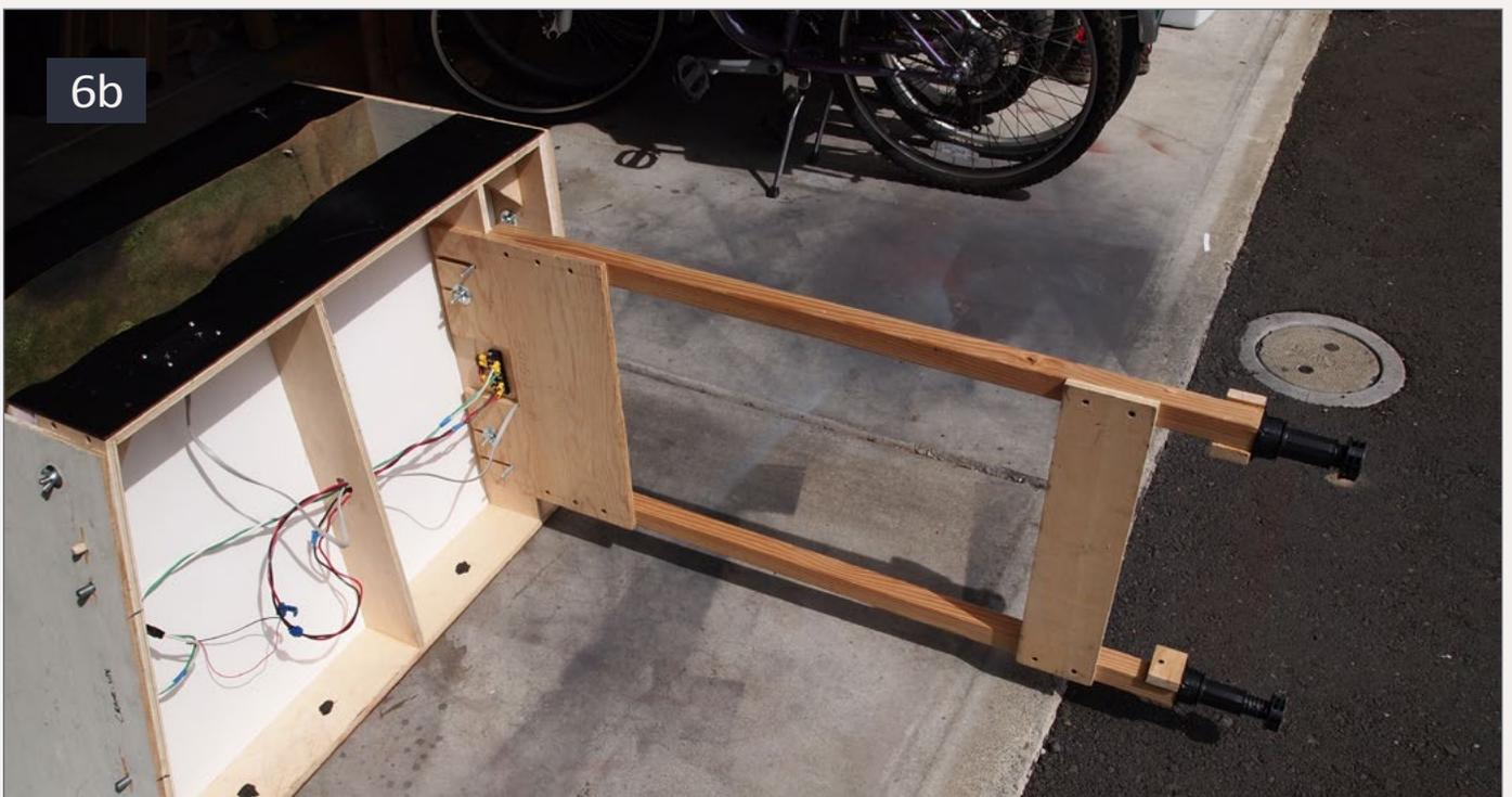
**6a-6b: Using  $\frac{1}{4}$ " bolts in T-nuts as leg levelers was cheap but operationally time-consuming and tiring. Rockler leg levelers are well worth the cost and are easy and quick to adjust.**
