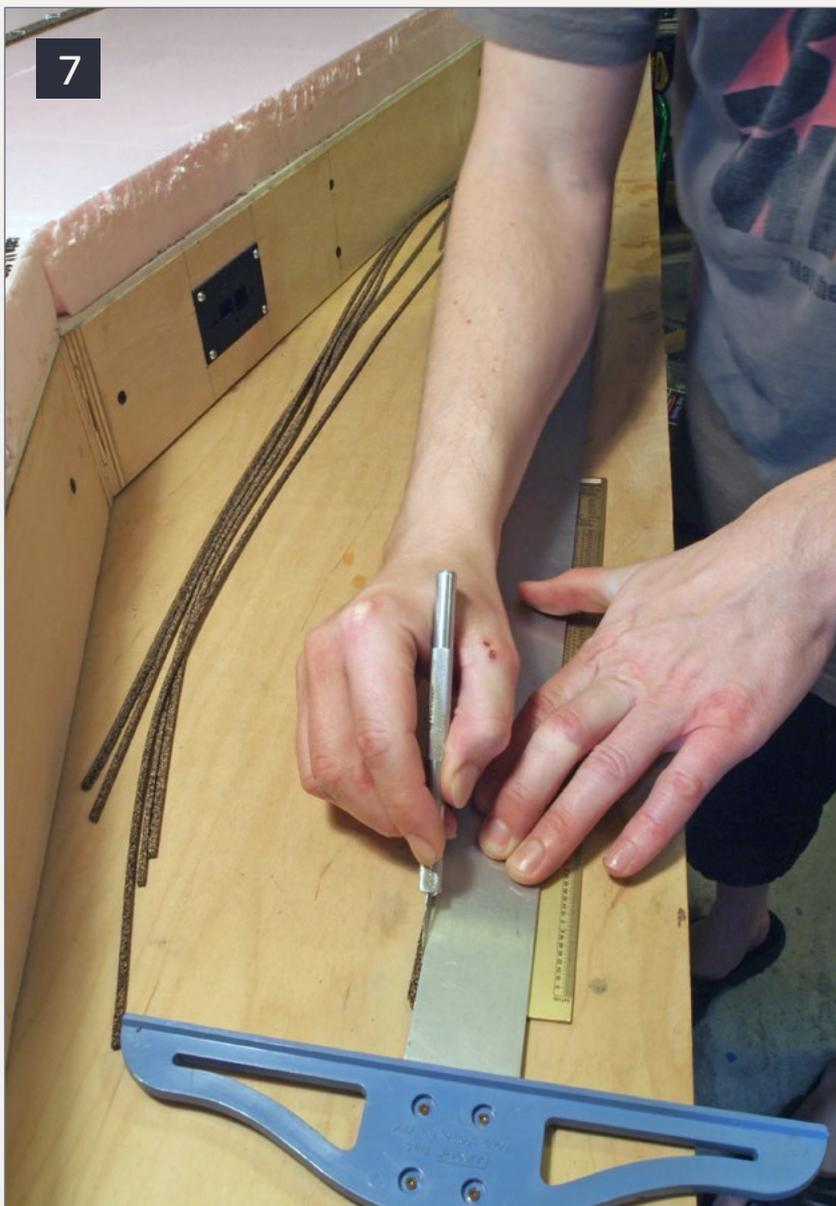
**7-8: Trimming about 1/8" off of the center of the cork roadbed strips gives the track a more branchline appearance. T-pins hold the cork in place while the caulk cures. The transition from roadbed down to ground was made by sanding down the pink foam into a sloping channel.**
