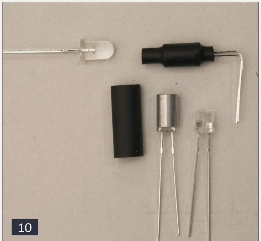
**10. Infrared switch components, LED on the left, phototransistor on the right.**
