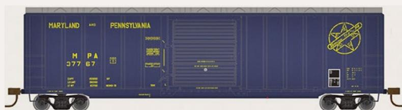
Atlas is quoting delivery in the first quarter of 2014 for this 50' Berwick boxcar. The Master® series model replicates a prototype built in 1972 with corrugated non-terminating ends and an X-panel roof. Models decorated for M&P (above), Canadian Pacific, East Erie Commercial, Railbox, and Wisconsin Central will have an MSRP of \$28.95. An undecorated model will be available at \$24.95.
