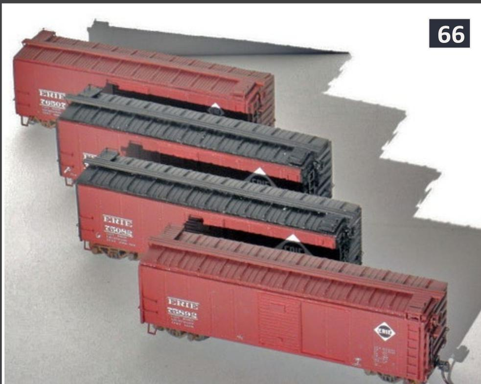
66: Next the running boards were cemented to the roof. After the main running board was cemented, I added the corner
