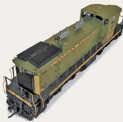
1200 horsepower road switcher built by General Motors in
