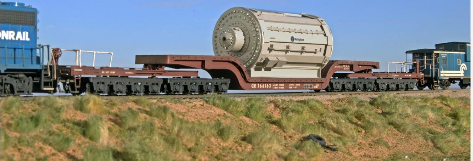
**7: This generator load is fashioned after prototype photos, to fit the brass Queen Mary depressed-center flat car. Lots of styrene and bolt castings were used to construct this model.**
