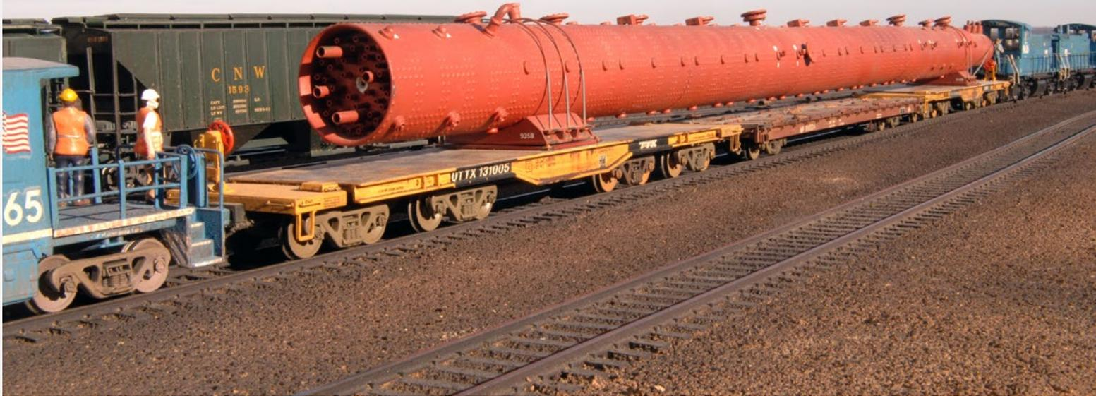
5: This small refinery fractionating tower is loaded on three flat cars. The outside flat cars bear the weight while the center idler flat keeps everything together during movements. The video shows the load running through a curve, illustrating the swing of the load and the cars in action.
