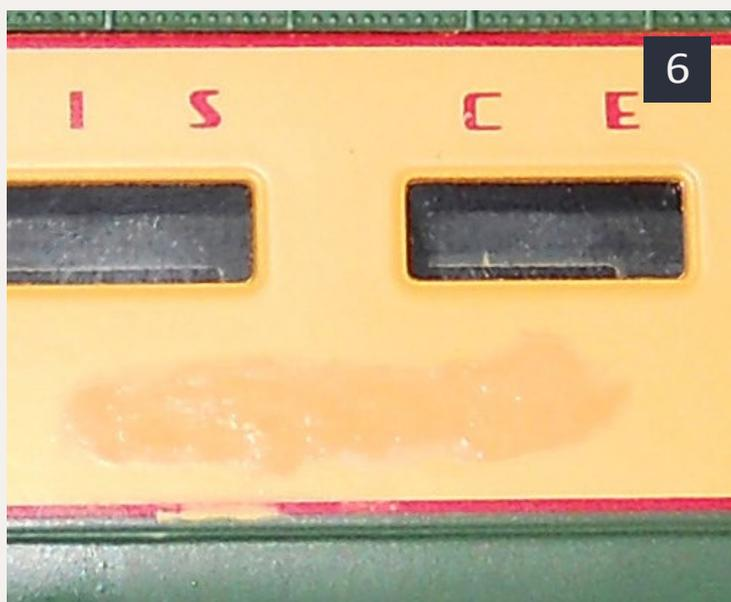
**6:.** The damaged paint. This is an example of one of the three cars that I tried to rename and renumber.
