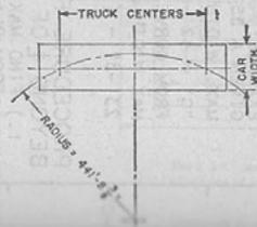
THE REDUCTION IN WIDTH IS PREDICATED ON THE BASE CAR, DEFINED ON PLATE C, AND ON A 13° CURVE.
