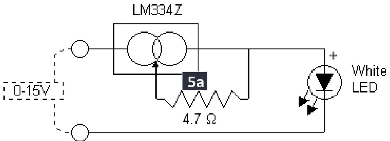
While most power supplies maximum is 12V this circuit can take as high as 20V
