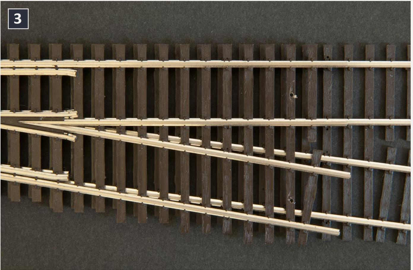
**3:** With a #6 switch sitting on top of a #8 switch, it's easy to see the difference in frog angles. The tips of the frogs are aligned. The #6 diverges at a greater angle than the #8, and the combination will not produce a smooth crossover if the two are installed face-to-face.
