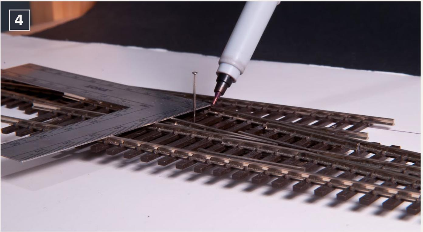
**4: Use your high school geometry to find the mid-point of a crossover by laying both switches in position and marking the mid-point of a line from the tip of one frog to the tip of the other. The distance is  $1 \frac{13}{16}$ " (46 mm), and using the diagonal line puts the shirt pin right in the center of the two rails.**
