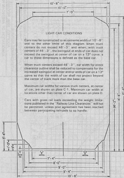
The 2'-3/4" above top of rail is absolute minimum under any and all conditions of lading, operation, and maintenance.
