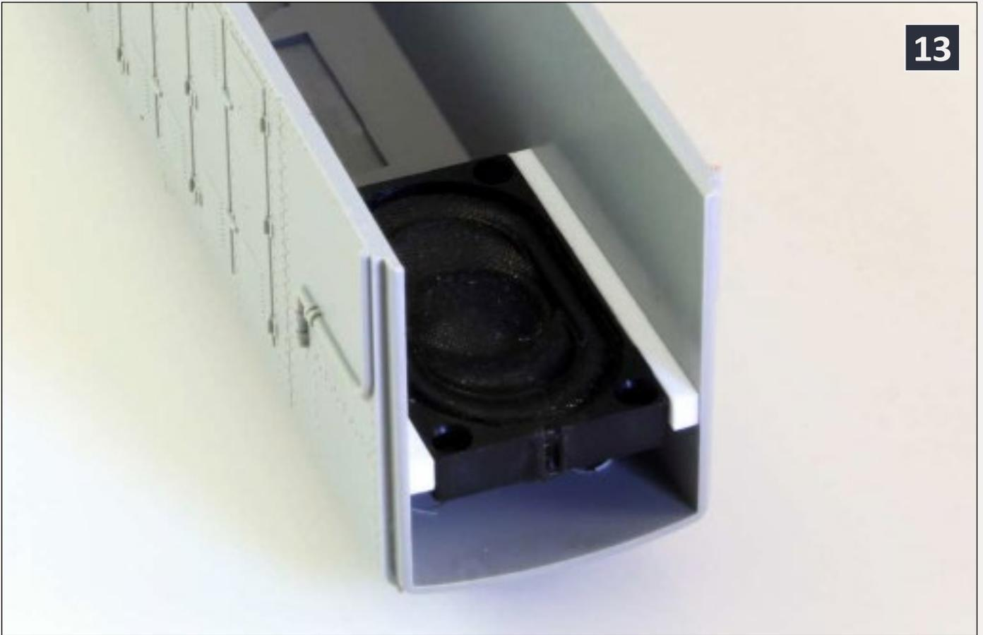
**13: The speaker is cemented into shell of the Atlas S-2.**
