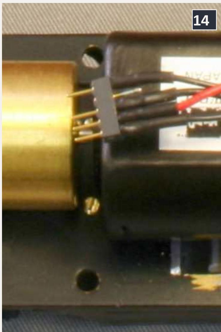
**14: This photo shows a connector with 3/64" shrink tubing on the connections, ready for an overall sleeve to insulate and stabilize the entire connector.**
