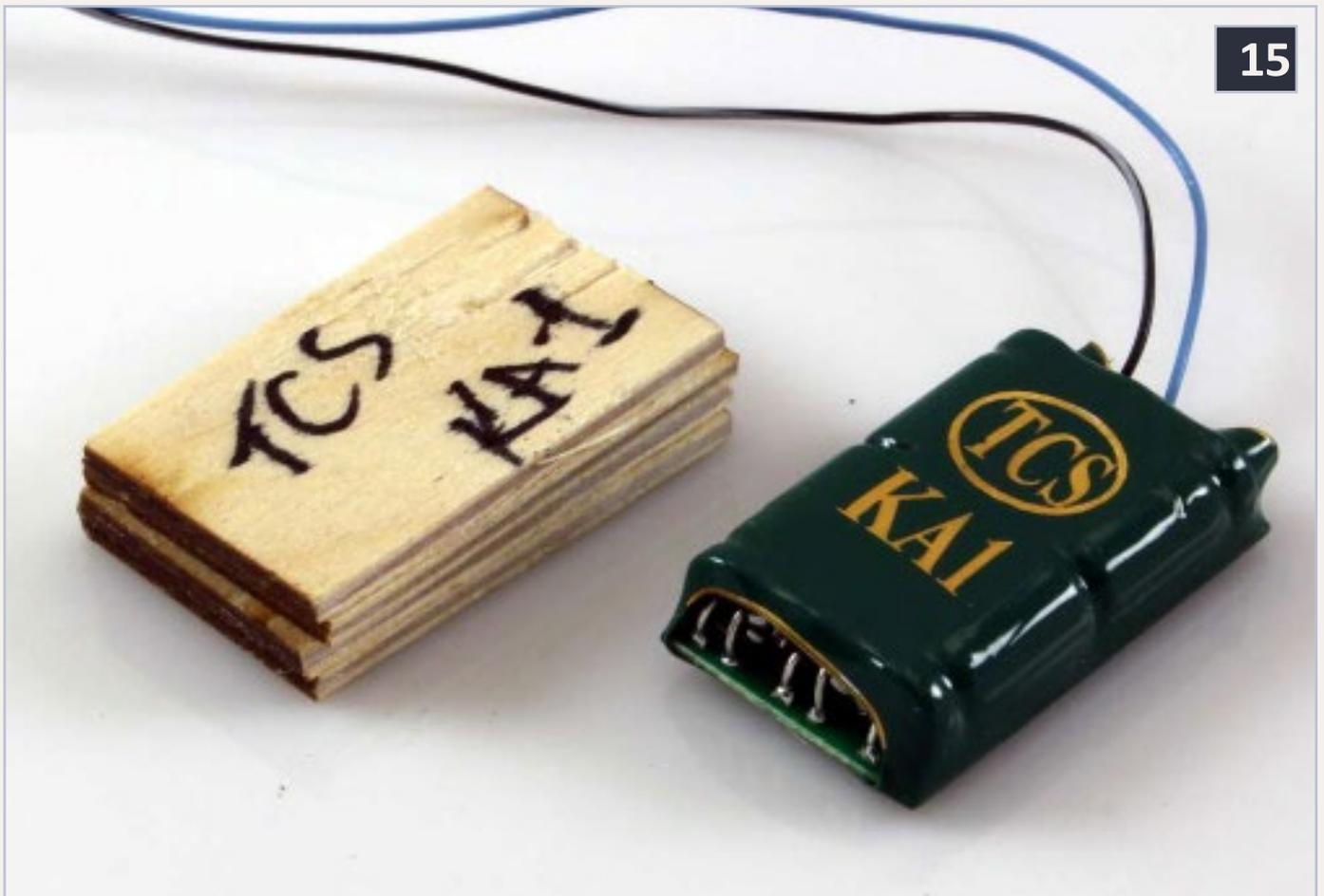
**15: This photo shows the mock-up I made for a TCS KA-1 and the actual part after I got it. I was able to verify that the KA1 would fit before I bought it with this mock-up.**
