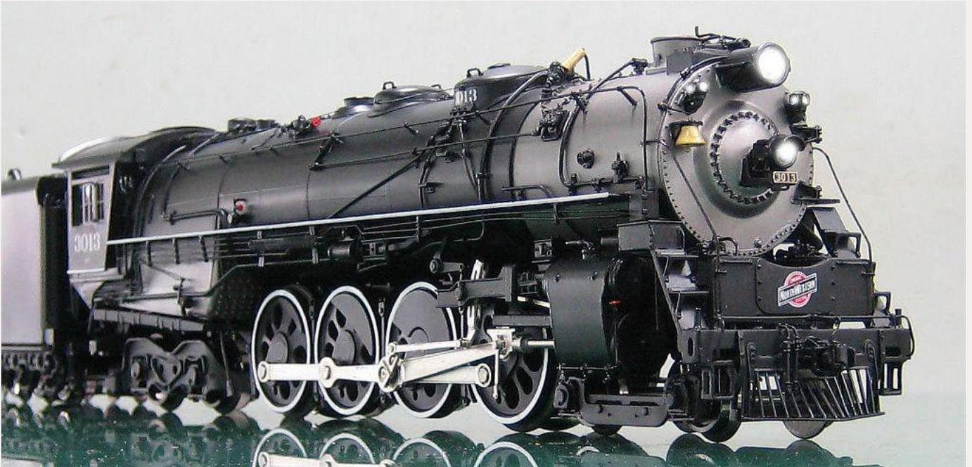
It was when the locomotives received numerous upgrades including new nickel-steel frames, new cylinders, and new fireboxes. They were redesignated as class H-1. The 4-8-4 Northern locomotives were assigned to both passenger and fast freight service, but because of their size and weight, CNW restricted them to the Omaha-to-Chicago main line. The models were handcrafted in Korea. Both 2-rail and 3-rail versions are available at \$1499.95 each.
