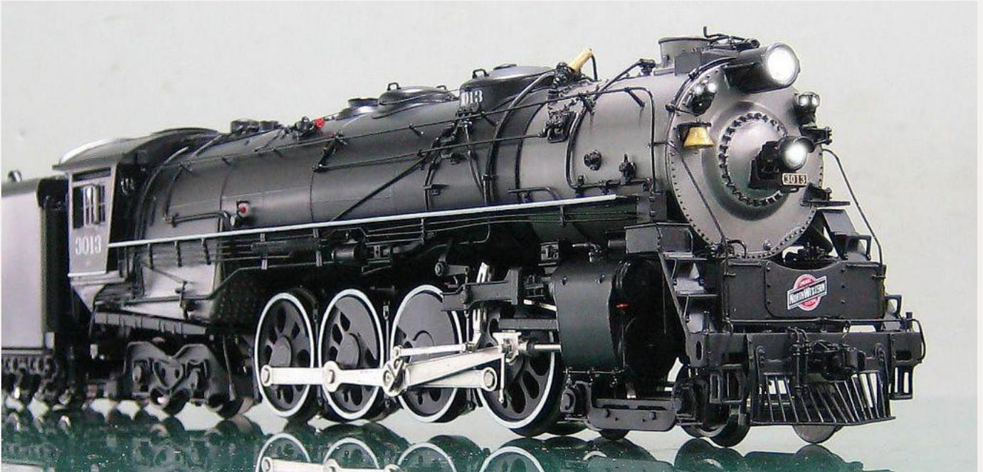
It when the locomotives received numerous upgrades including new nickel-steel frames, new cylinders, and new fireboxes. They were redesignated as class H-1. The 4-8-4 Northern's were assigned to both passenger and fast freight service, but because of their size and weight, CNW restricted them to the Omaha-to-Chicago main line. The models were handcrafted in Korea. Both 2-rail and 3-rail versions are available at \$1499.95 each.
