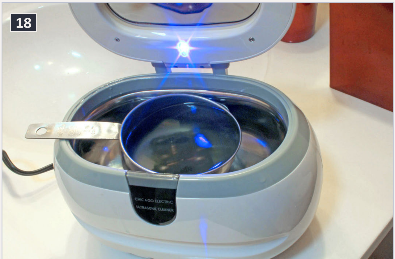
18: Cleaning drive train parts in ultrasonic cleaner.
