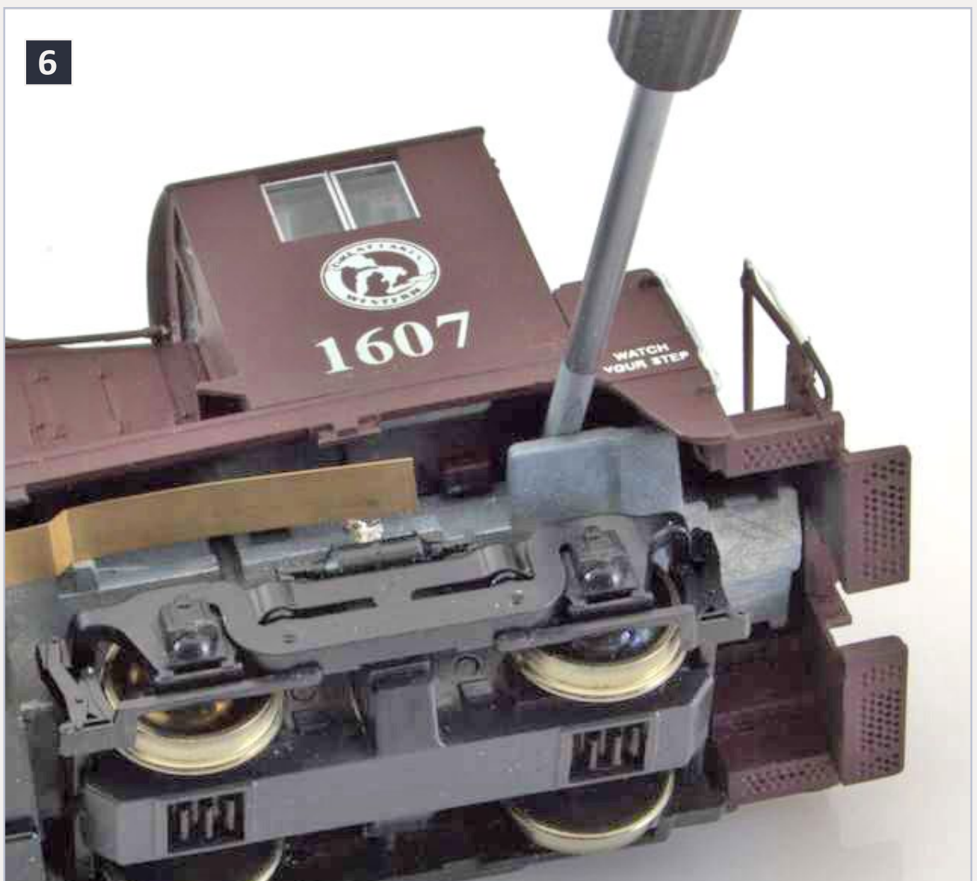
6: Prying the shell off the frame.
