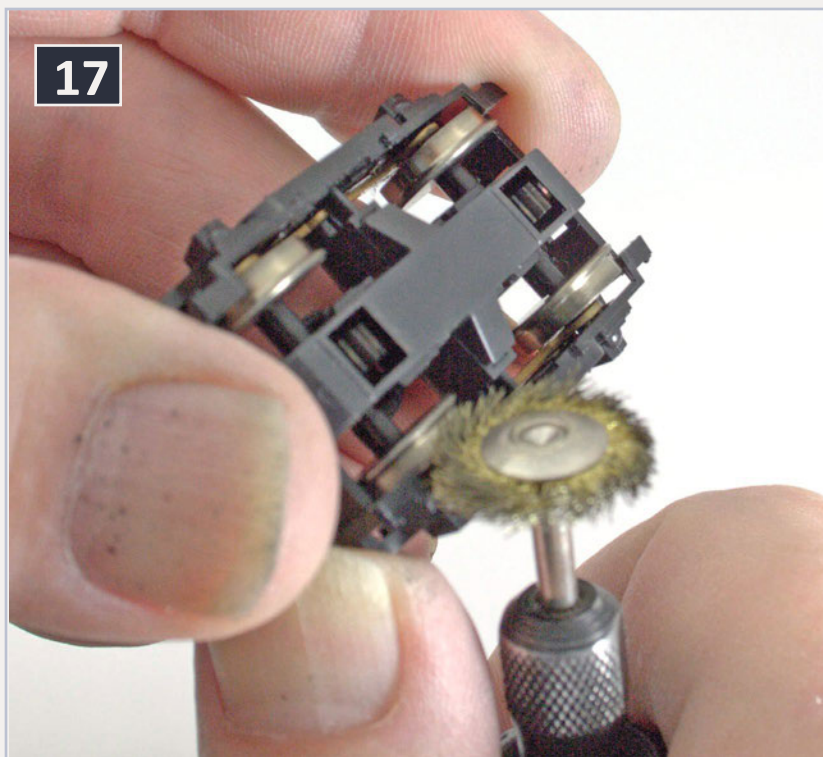
17: Cleaning the truck assemblies with a motor tool and brass brush wheel.
