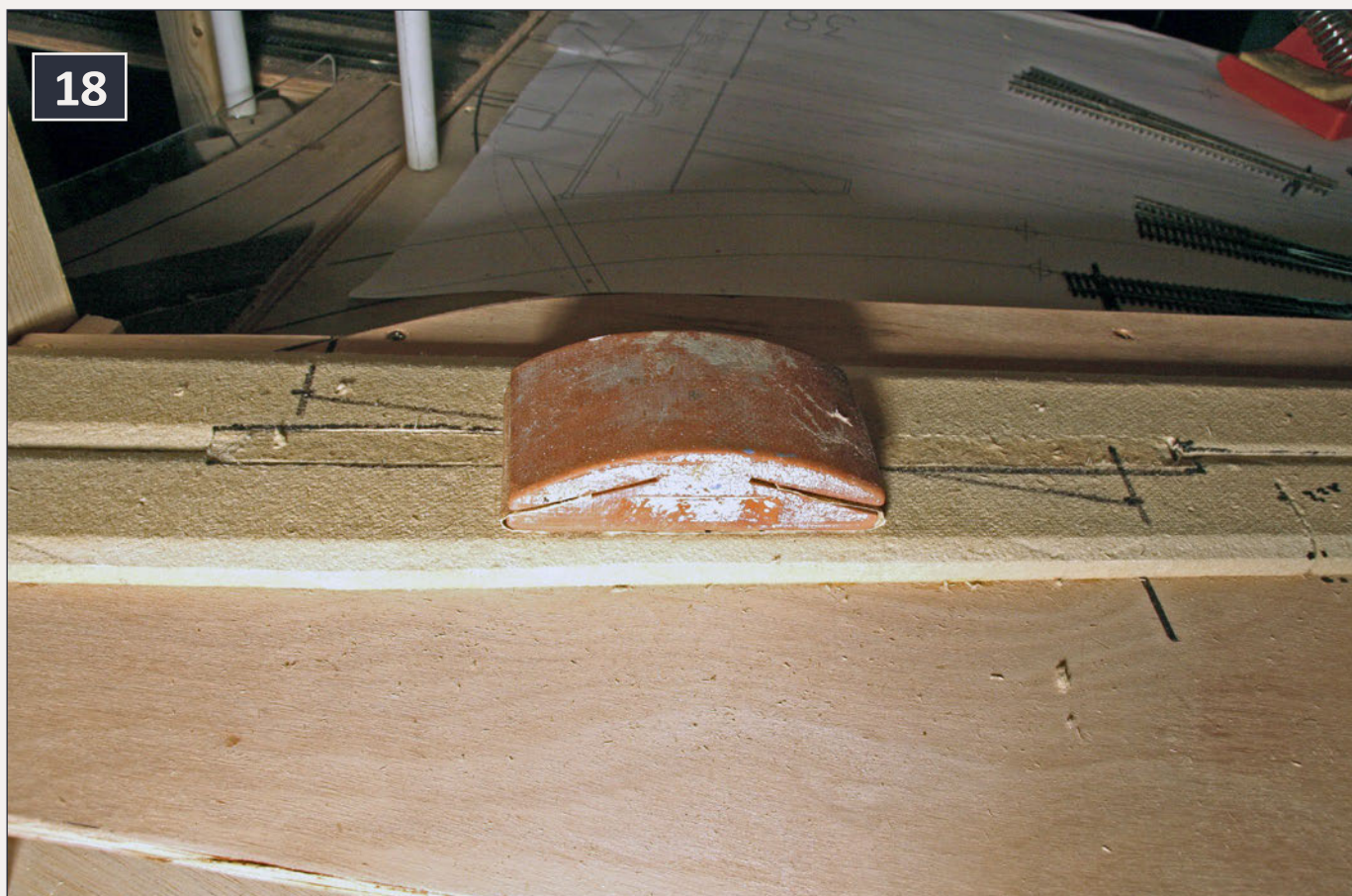
18: Sand the roadbed top smooth.
