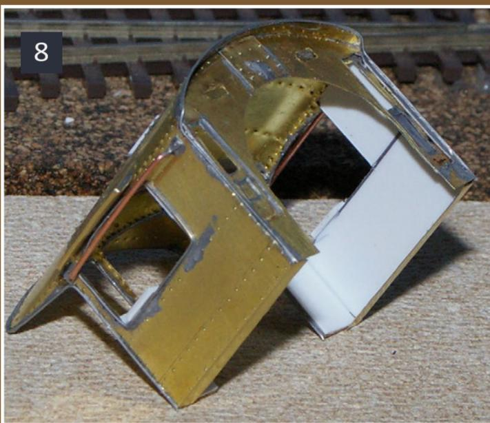
8: I added styrene to the inside of the cab to hide the back sides of the rivets. It also simulates the wooden window frames.
