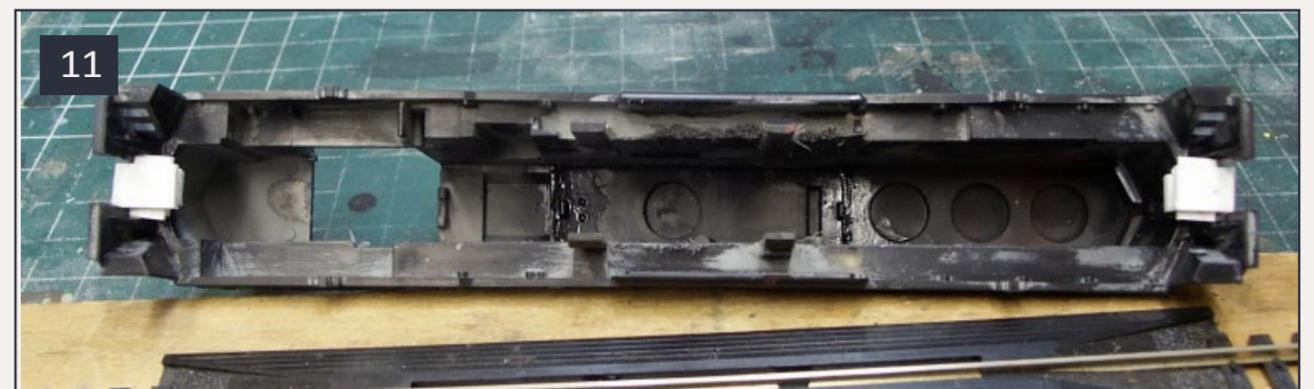
**11:** Loco shell, with the new styrene coupler pads to allow body-mounting the couplers.
