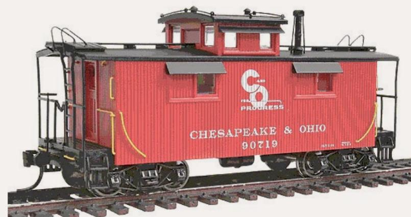
Walthers new Proto 25' C&O wood caboose is available now at \$39.98. Four different paint schemes are offered on the HO scale ready-to-run model that is based on C&O 90700 series cabooses that were built in the 1920s and remained in regular service through the 1960s.
