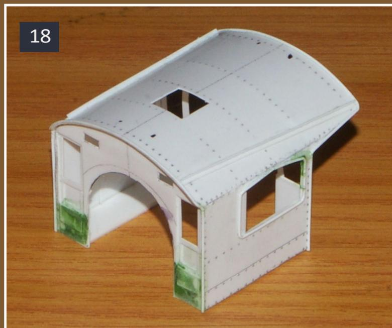
18: Here you can see the hole in the roof for the ventilator, as well as the gutters, the floors, and the patched doors.
