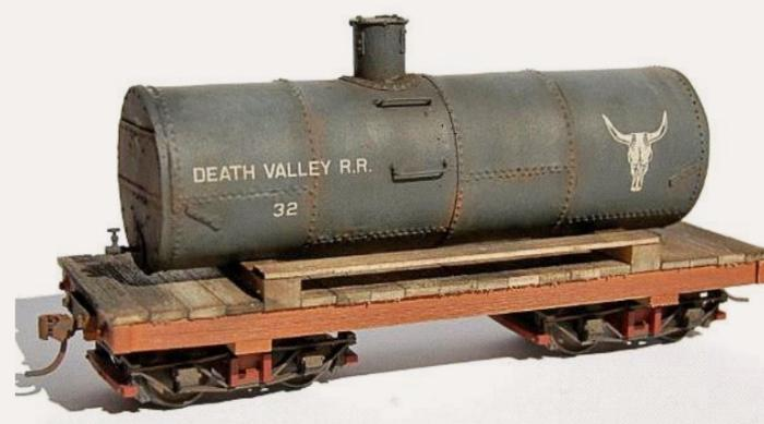
Morgan Hill Models ([morgan-hillmodels.com](http://morgan-hillmodels.com)) is selling a kit that builds into an On30 20' Tank Car. The tank and car frame are cast resin. Basswood is supplied for the deck and tank supports. Suggestions for painting, staining and weathering are included with the kit that sells for \$34.95.
