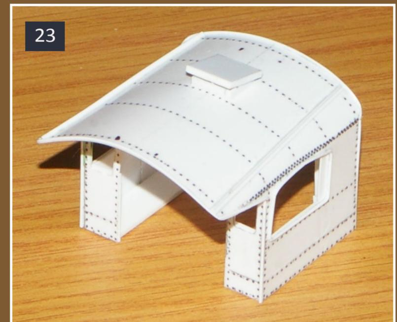
23: The rear of the finished cab. The rivets over the cab window are tank car seam rivets, while the rest are individual strips.
