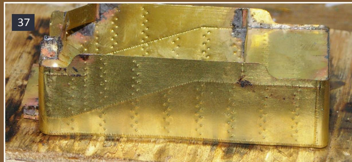
37. Here is the tank, right after soldering the pieces together. It helps having a sacrificial piece of wood to work against.
