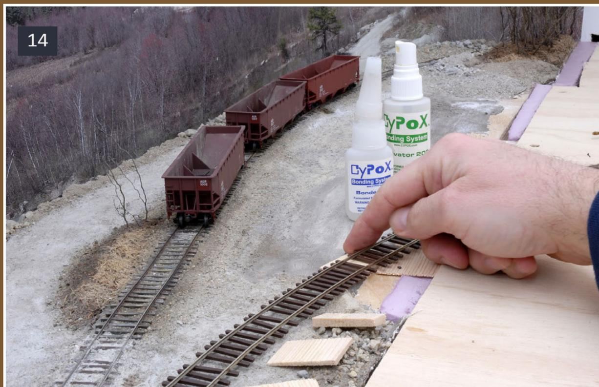
13: It was now time to permanently install the quarry siding. I started by removing ties from my flex track with a rail nipper. I like to remove every 6th or 7th tie. This thins the tie density on the flex track, which is important to differentiate secondary sidings and industrial tracks from main line track.
