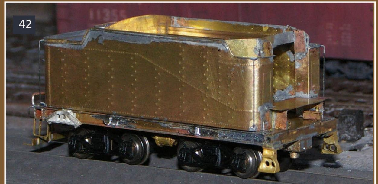
41: The tank should sit nice and flat on the frame. The two are not attached in any way in this photo. The front of the tank is open, to provide an opening for the speaker to be heard through.
