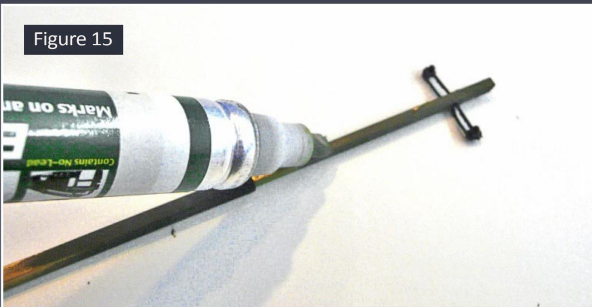
Figure 14: I slipped the sign post down the larger tube, and then painted the whole assembly a dark gray automotive primer. I “masked” the LEDs with bits of tape, then came back and brush painted them with PollyScale Tarnished Black, which is close to the color of the spray paint.
