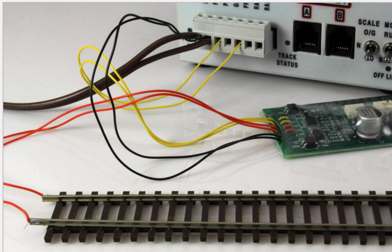
Figure 11: Digitrax DCS100 connected to a PTB100.
