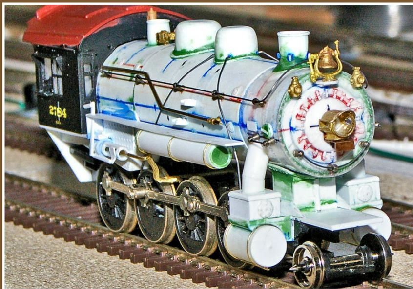
Figure 14: The smokebox detail parts are installed, along with the handrails.
