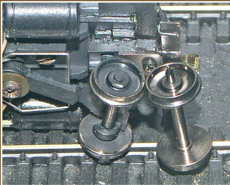
Figure 25b: Finished pilot wheels after modifying the axles.
