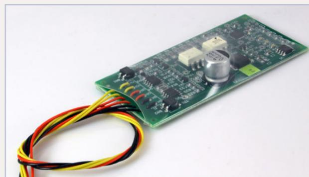
Figure 9: SoundTraxx' PTB100 Programming Track Booster.
