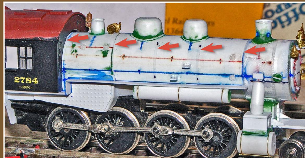
Figure 8: While they are difficult to see (marked with red arrows), the lagging bands have been added. The black marks on the boiler were used to get the correct spacing.
