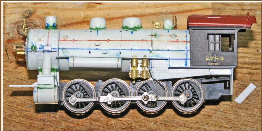
The pop-valves are made from the same tubing and rod used to make the clean-out plugs in the boiler. The tubing should be just over half the inside diameter of the turret. Cut
