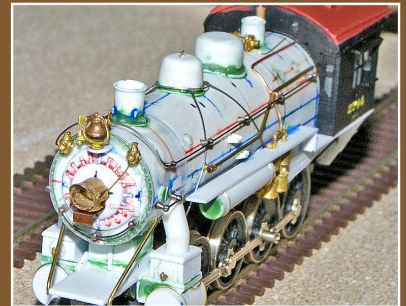
Figure 15: The power lines have been run to the headlight and marker lamps.
