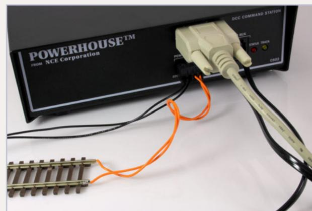
Figure 5: NCE command station with RS232 cable interface.
