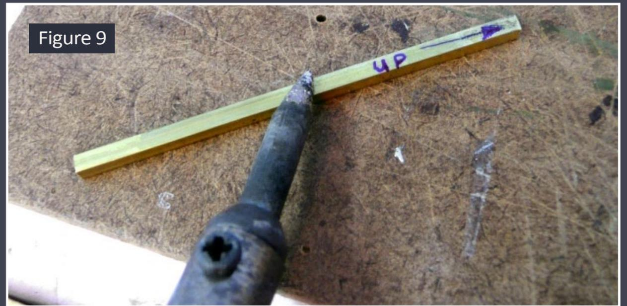
With both LEDs prepped, I began work on the sign post and mounting base. I cut two lengths of 3/32" tubing, one 2-1/2" long and the second about 1". I also cut a 3" length of 1/8" tube. The 1/8" tube will be the base of the sign post, and since this will form part of the conduction path for the common lead, it has to be long enough to extend below the layout. My benchwork is 2" extruded foam glued to 1/2" plywood, so I cut my base tube 3" long, but this will vary for other types of benchwork.
