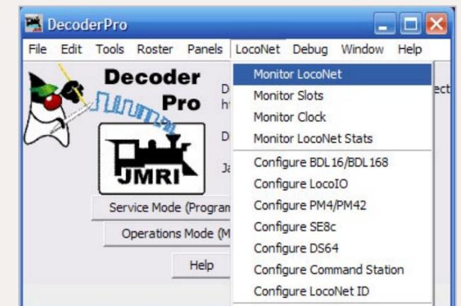
Figure 8: DecoderPro Screen shot with Monitor LocoNet selected.
