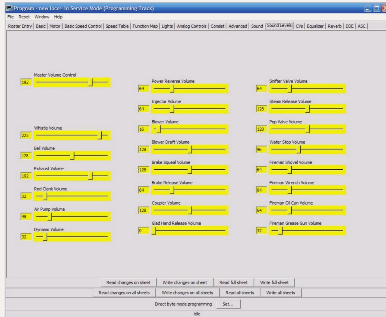
Figure 12: Tsunami Sound level page in DecoderPro.
