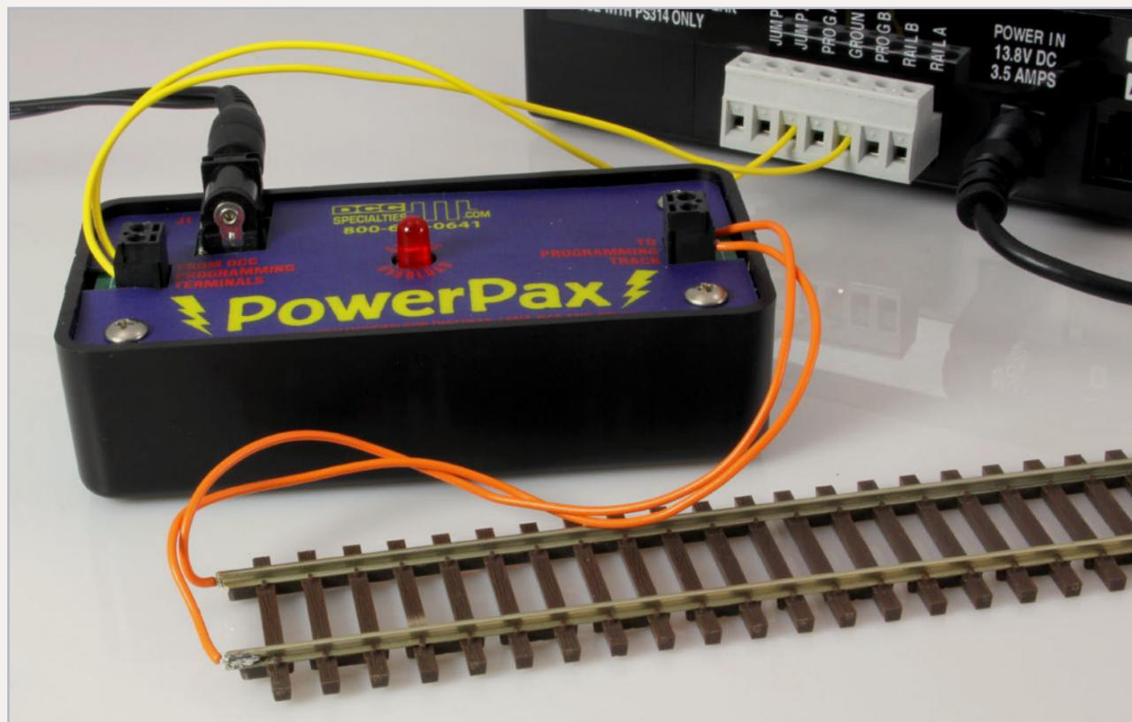
Figure 10: Digitrax' Zephyr connected to a PowerPax PTB.
