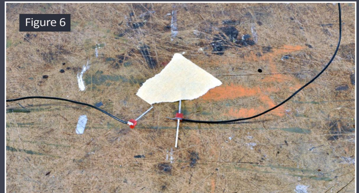
I started by using my ohmmeter to identify which lead on my LEDs was the positive (anode) and which was the negative (cathode). Because the common terminal on the FL-2 is positive, I had to make sure I solder the positive anodes of both LEDs to the brass mast for my flasher to work.
