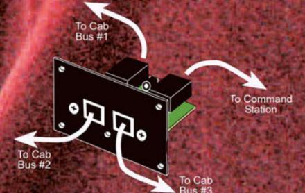
You can use a UTP panel as a three way "Y" splitter and go two or even three ways with your Cab Bus!
