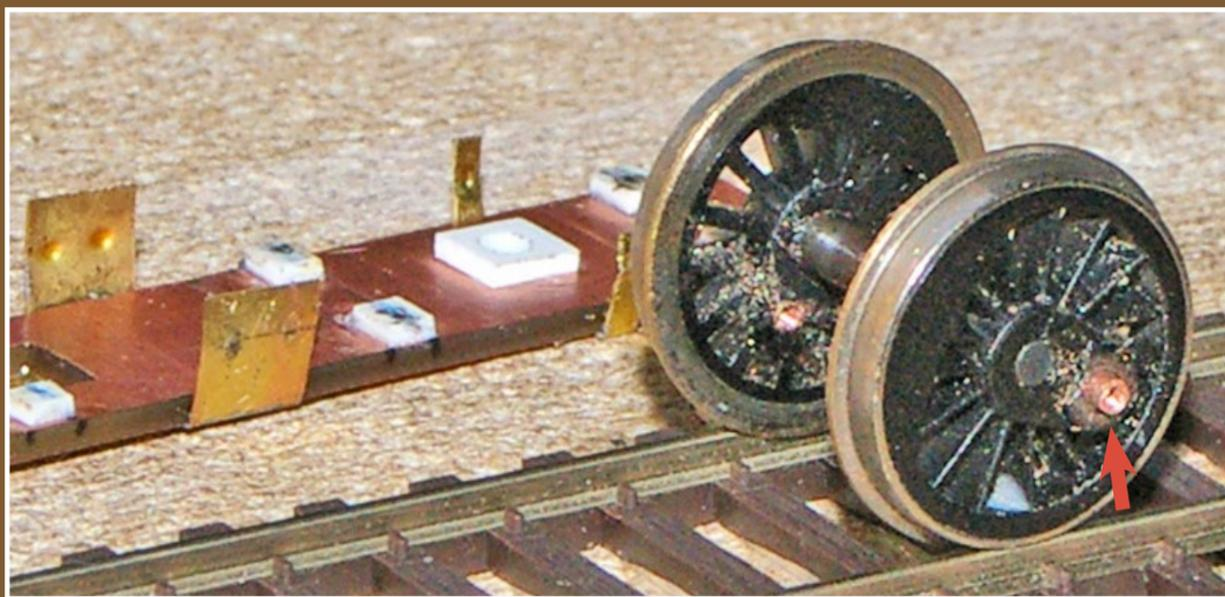
Figure 26: I made new crank pins from 1/16" copper tubing (red arrow). It just happened to slip into the original crank pin holes with almost no modification, and it's the perfect size to drill and tap for a 00-90 screw.
