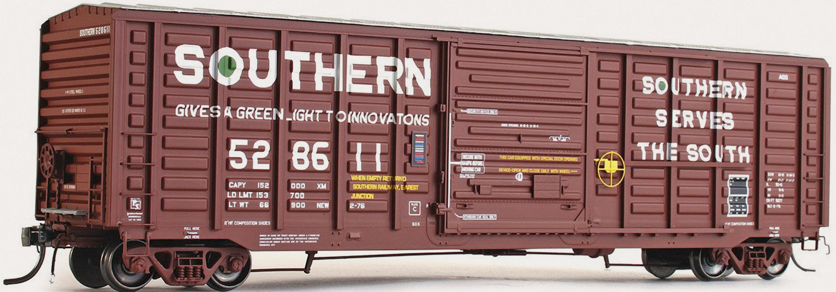
Southern Railway's car number 528611 epitomizes the rugged 60' waffle-side boxcar seen all across America. ExactRail has produced **HO scale** models of the Pullman-Standard 7315 cu. ft. car in several additional schemes including L&N, NW, BNSF, DT&I, CSXT, ATSF, Milw Rd, NS, UP, and GTW.
