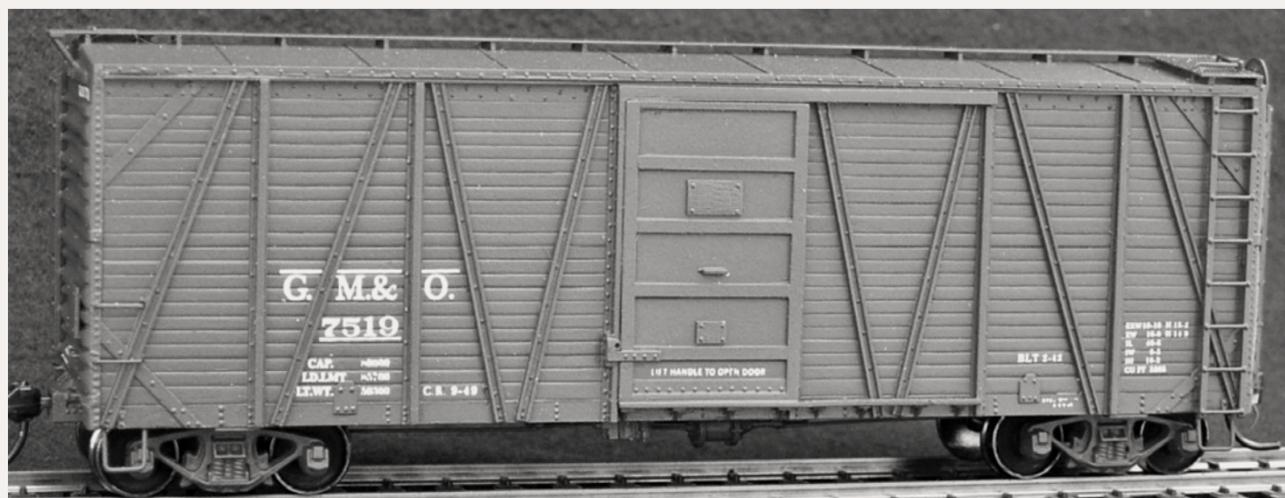
Sunshine also has the 10'3" ACY and GM&O cars with improved Dreadnaught ends and Pullman steel doors (above), as upgraded on the prototype beginning in the mid-1940s. Sunshine kits come with extensive instructions and a prototype data sheet, proprietary decals and all necessary detailing parts except trucks and couplers. They are priced at \$42.00 each.
