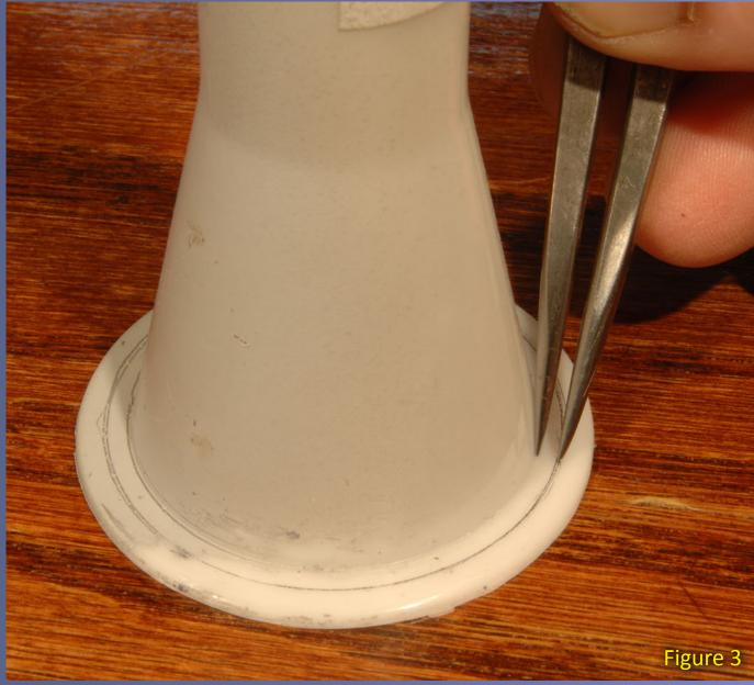
Figure 3: The flange on the stuffing tube was too wide to look right. I used a divider with sharp points to measure and scribe the flange to remove about  $\frac{1}{8}$ " around. This leaves about a 7 scale inch flange for the bolt holes.
