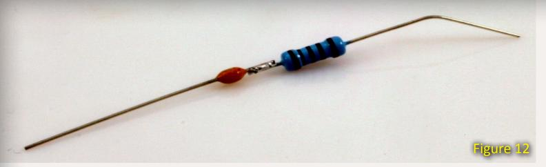
Figure 12: A snubber made from a 100 ohm 1/2 watt resistor and a 0.1  $\mu$ F 50 volt or higher capacitor.
