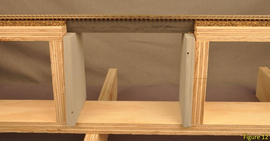
Figure 11: Holding the bridge abutment height fixture tightly to the subroadbed helps vertically align abutments. Hot glue works well to attach the gray abutment to the plywood abutment riser – it sets almost instantly!
