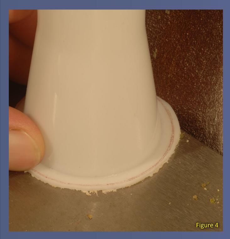
Figure 4: I used a table mounted disk sander to very carefully remove the flange outside the scribe line. You must keep the curvature even and smooth or it won't look right.
