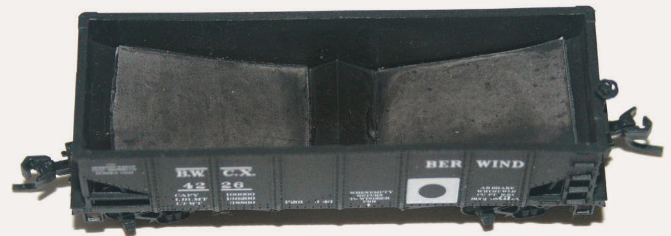
Figure 3: Sheet lead fitted to the slope sheets of a 2-bay hopper. Further weathering will disguise the appearance of this material.
