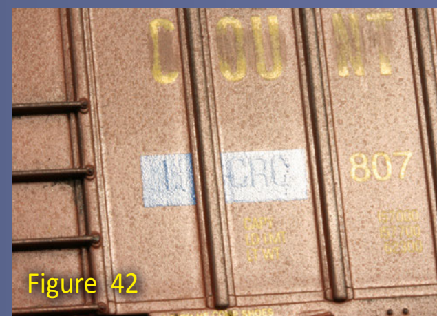
Figures 42-43: An interesting effect can be created by placing trim film directly over factory printing that has not been made smooth with the paint surface. The relief of the raised printing will show through the trim film, leaving a ghost effect such as the 'BIG BLUE' showing through on this ex-CSX boxcar.
