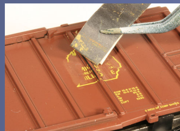
Figure 31: Thin sandpaper can become very rigid and allow excellent control when it is cut into thin strips and folded over upon itself.
