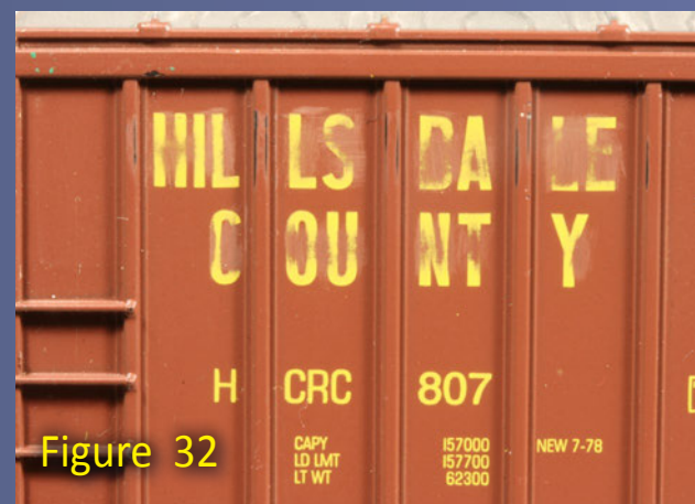
Figures 32-33: Varying the amount of distress of the car's graphics can create the look of aged, faded, or flaking paint.
