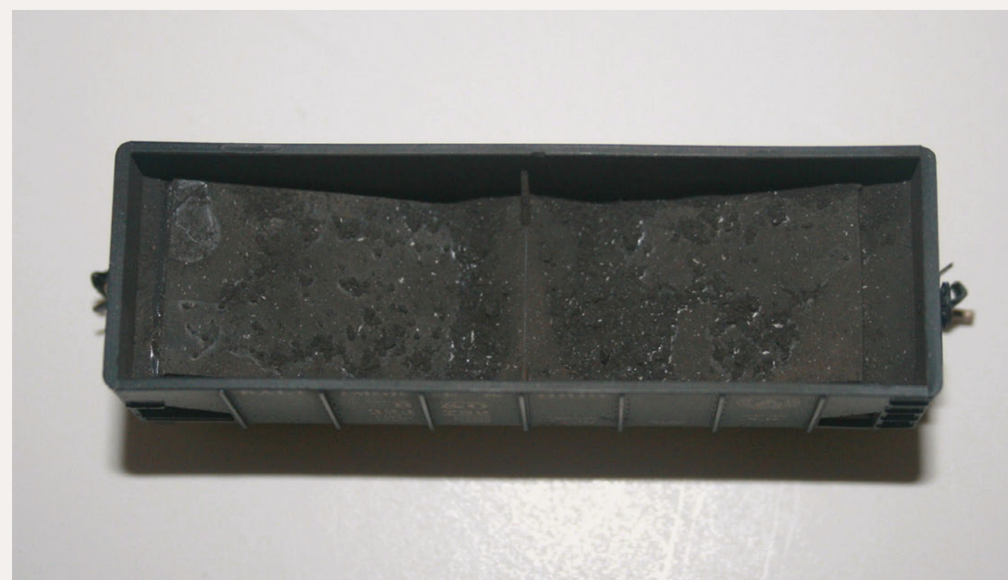
Figure 7: This overhead view shows a 2-bay hopper with sheet lead on the hopper bottom, grimy black and rusty weathering, and the remains of the previous coal load. The coal and weathering almost completely hide the added weight, even from this angle.
