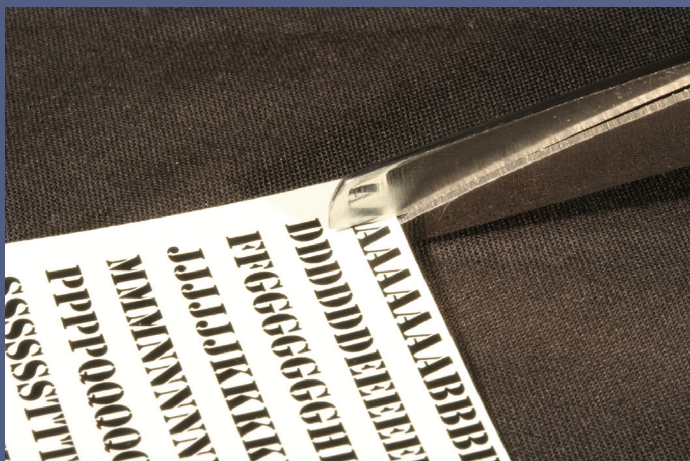
Figure 44: Decals printed onto a solid sheet of clear film should be trimmed close to the printed characters, leaving a minimum of clear film surrounding the characters.
